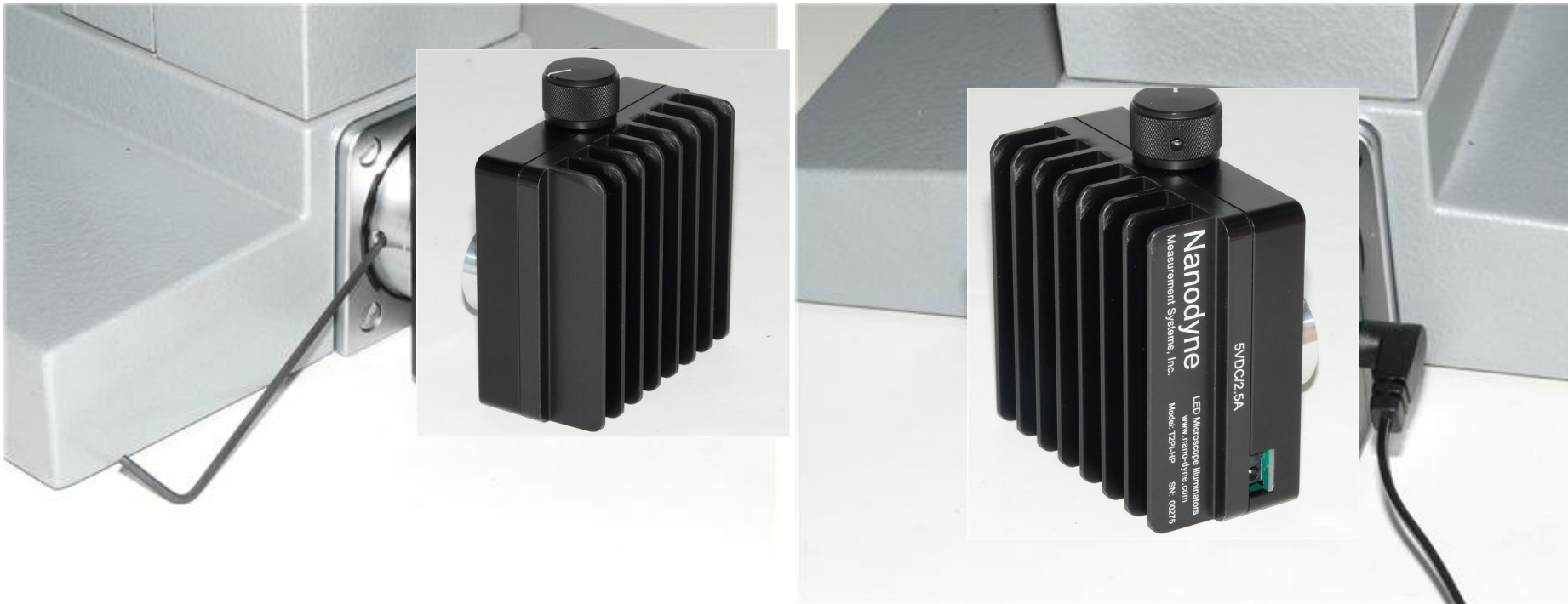
Step 3: Tighten the original screws to secure Nanodyne adapter in place.
