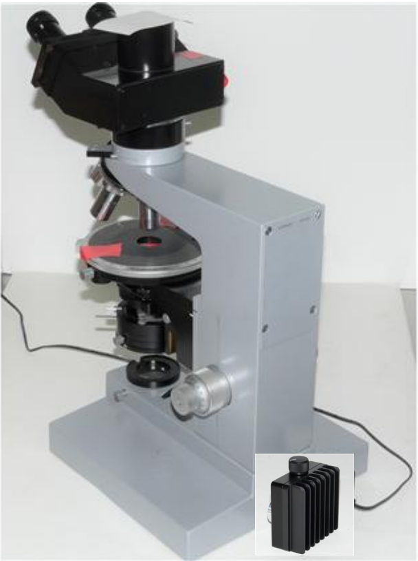
Step 4: Tighten the set screw to secure Nanodyne illuminator in place, (only in the case of remote adjustment pot) connect the pot cable, and secure the cables using 3M VHB tape if needed. Plug AC adapter to the Nanodyne illuminator and now it is ready to use.
