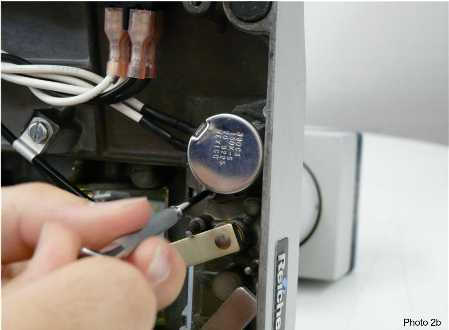
Locate the potentiometer that controls the light intensity underneath the microscope and remove the plate holding it in place with a screwdriver. Keep the plate for future use.
