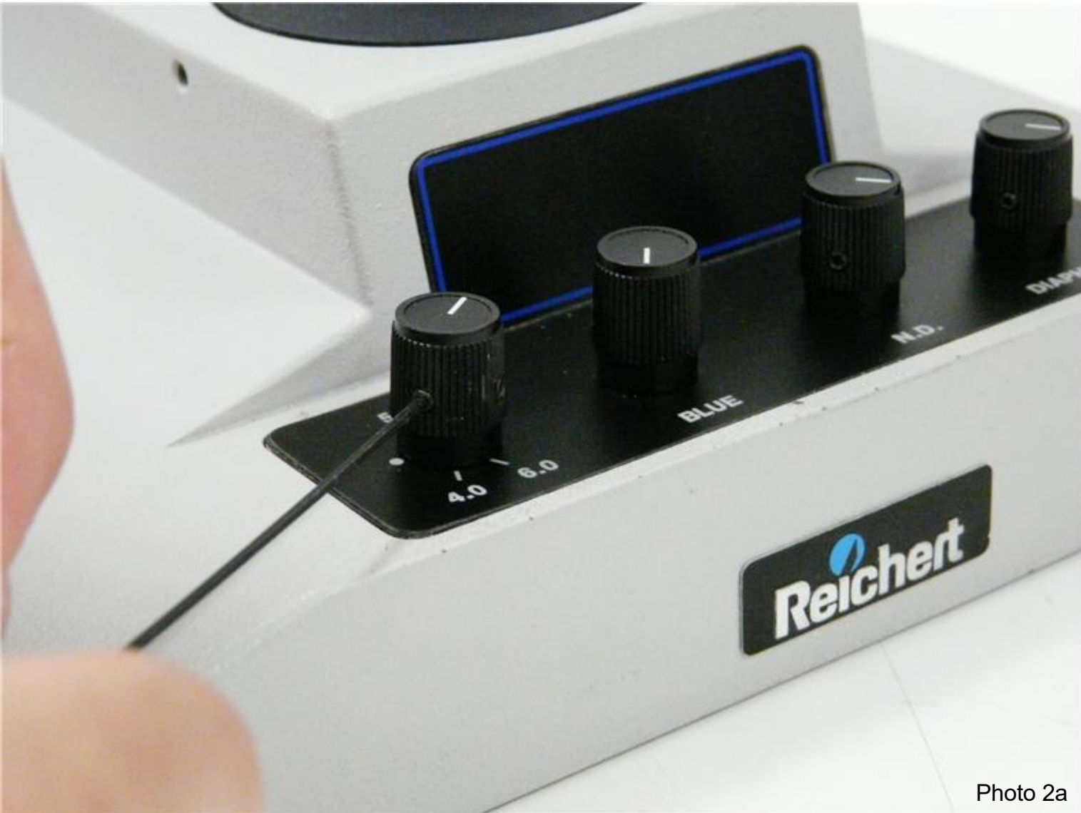
Using the hex key provided, remove the set screw holding the brightness dial in place on the top of the microscope.
