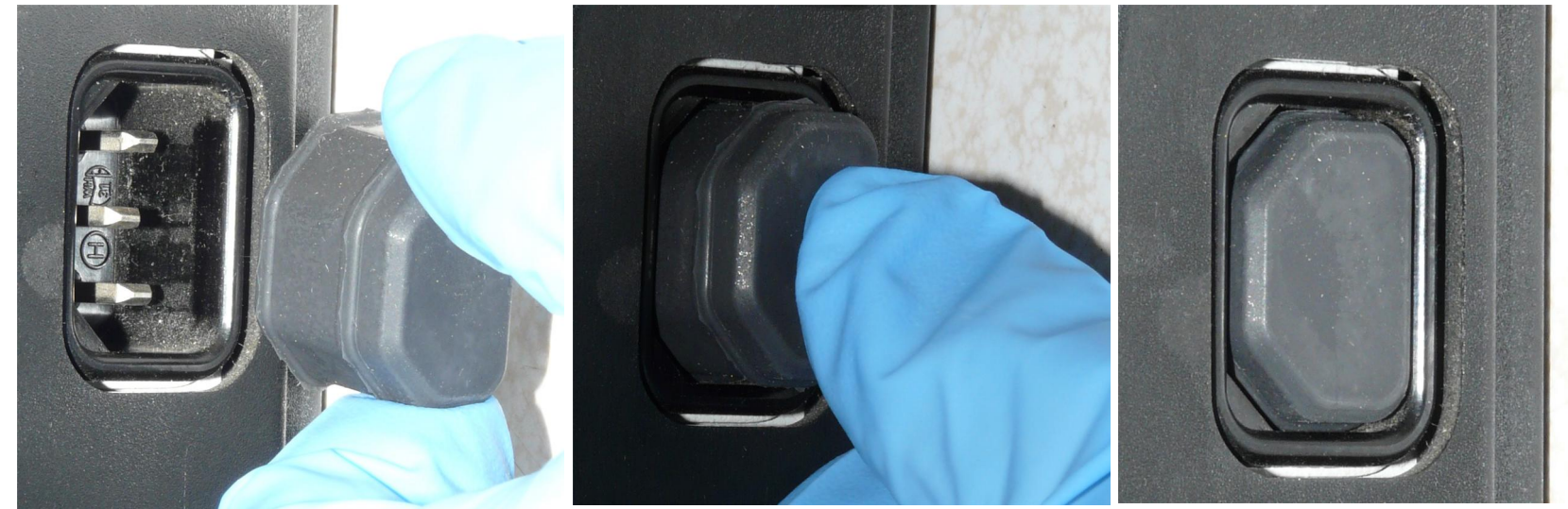
Installation of PN 10736 rubber plug to deter connection of obsolete AC power cord.
