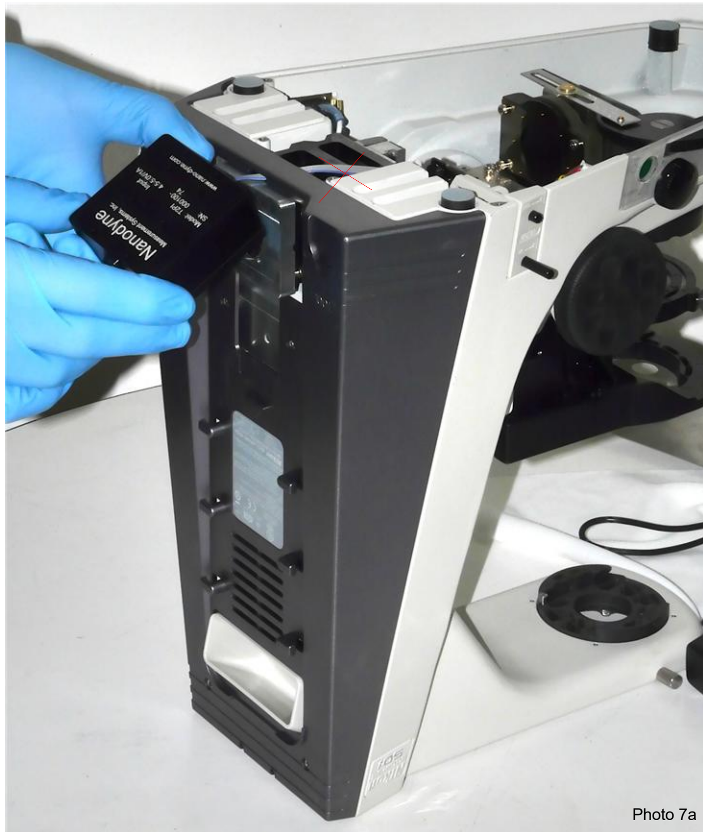
Routing the Nanodyne pot cable through back cover of microscope.
