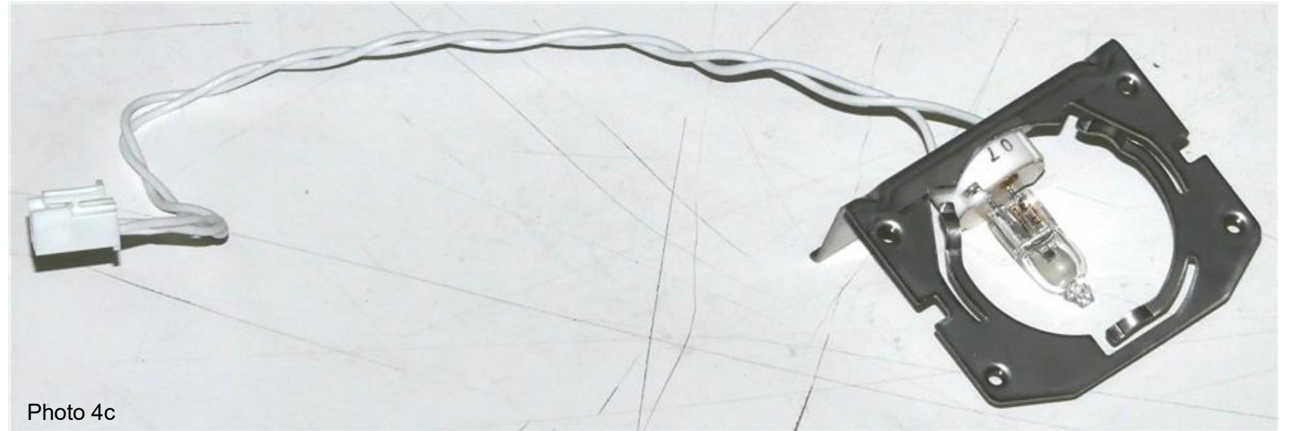
Photo 4c Original lamp plate and cable removed from microscope.
