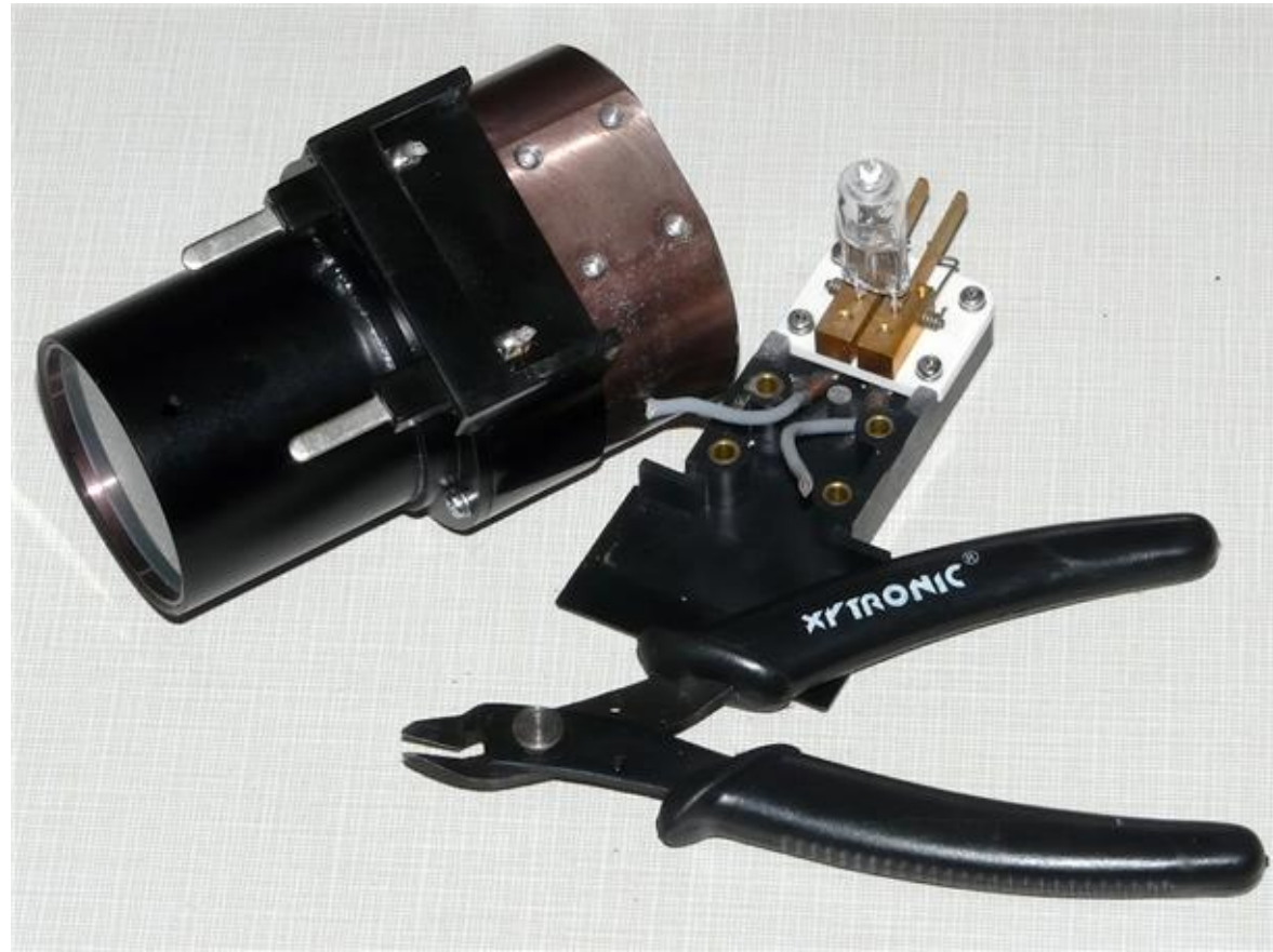
Step 3c) Cut the wires close to the condenser lens to remove the lamp holder. The lamp holder may be discarded. (photo at left)
