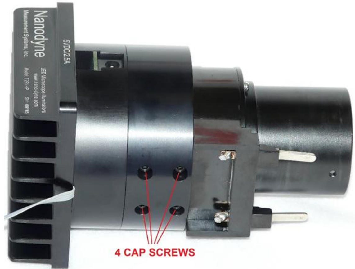
Step 4) Insert the original Olympus condenser lens assembly into the Nanodyne illuminator assembly, and secure with the four M3 x 0.5 x 8mm cap screws provided, using the provided 2.5mm hex key to tighten securely. (photo at left)
