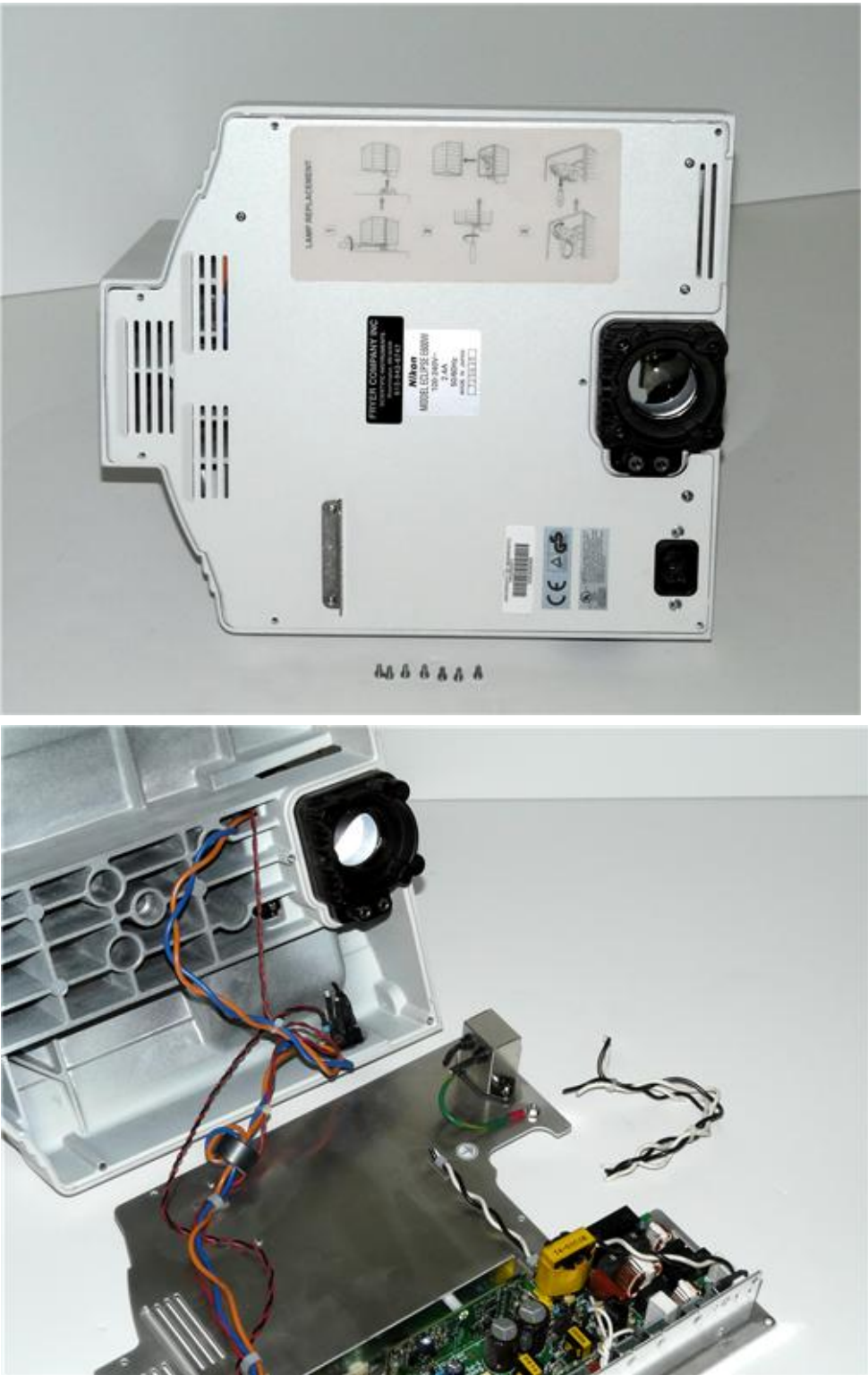
STEP 2: Remove the old illuminator, and then remove the back plate of the microscope by unscrewing the screws that hold it in place.
