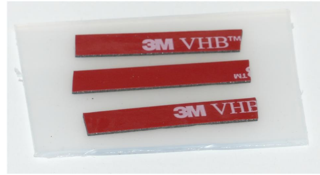
Tape to secure wires.
