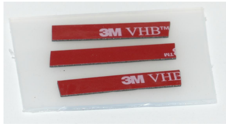
Tape to secure wires.
