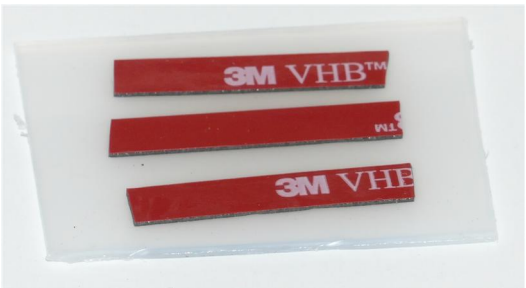
3M VHB tape to secure pot cable
