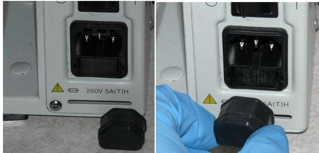
Installing PN 10736 rubber plug in AC receptacle to deter connection of obsolete AC power cord.
