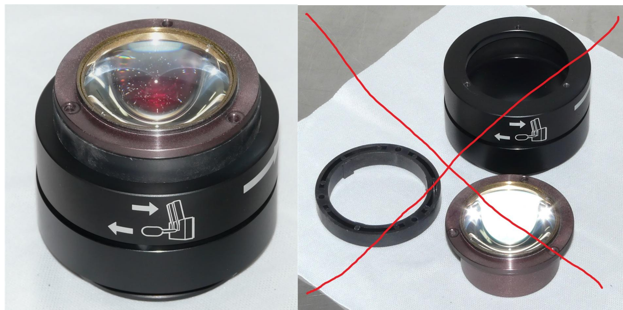
(2) Don't let the collector lens fall out of the housing after removing the screws.
