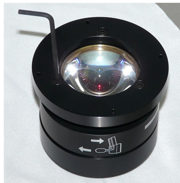
(4) Attach the adapter to the collector lens using the three 25mm long M3 screws. Tighten with the included 2.5 mm hex key.
