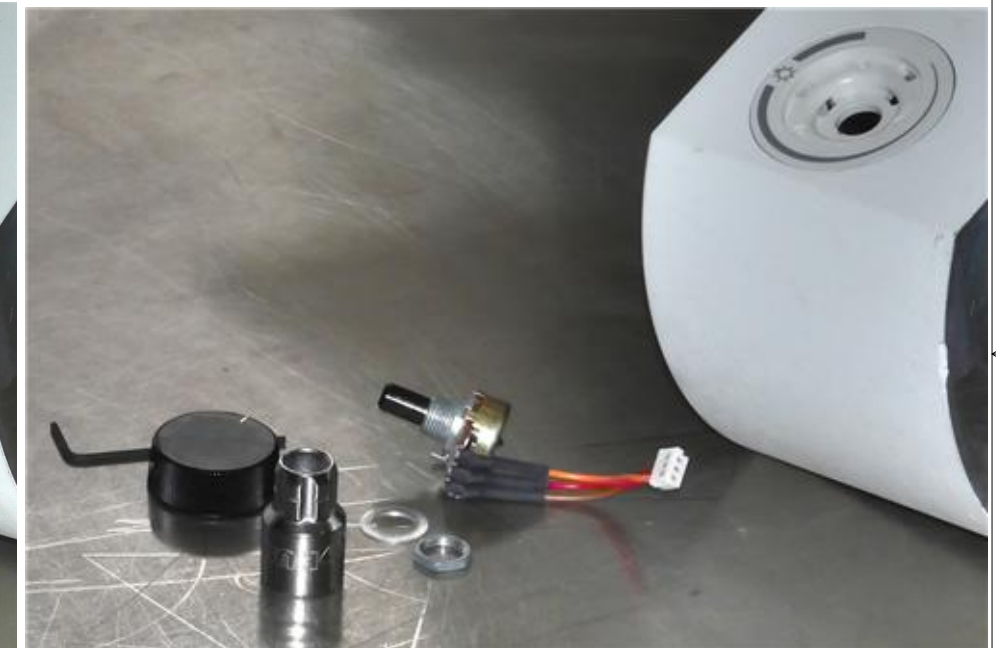
(3) Remove the knob from the adjustment pot using the 1.5mm hex key. Then remove the nut holding the pot with an 11mm socket. Remove the pot and the attached cable. It is not necessary to remove the cable from pot.
