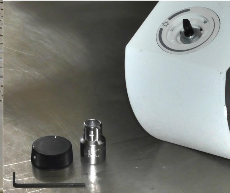
(3) Remove the knob from the adjustment pot using the 1.5mm hex key. Then remove the nut holding the pot with an 11mm socket. Remove the pot and the attached cable. It is not necessary to remove the cable from pot.
