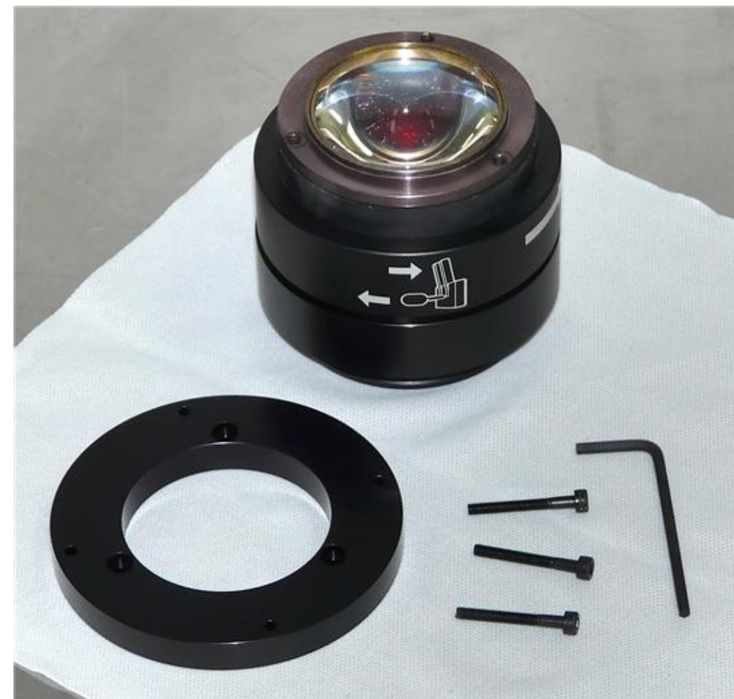
(3) Ready to attach adapter to collector lens assembly.
