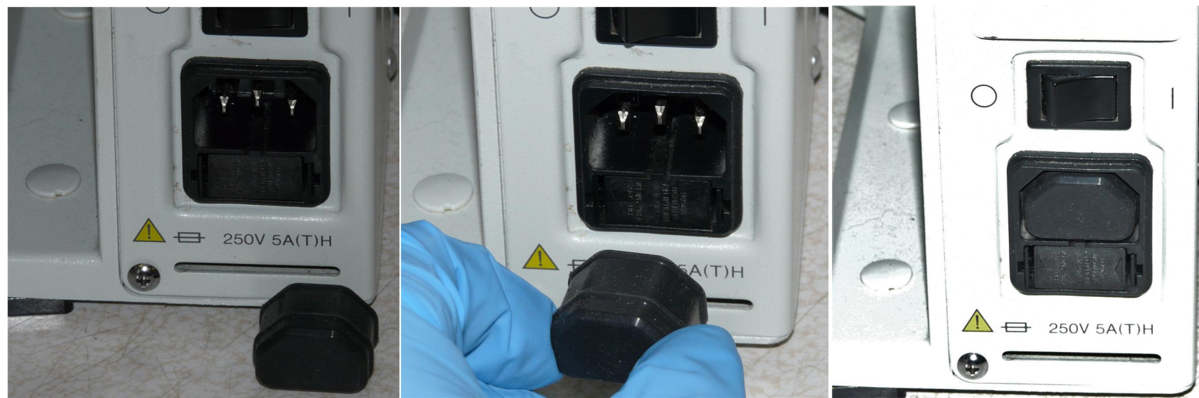
Installing PN 10736 rubber plug in AC receptacle to deter connection of obsolete AC power cord.
