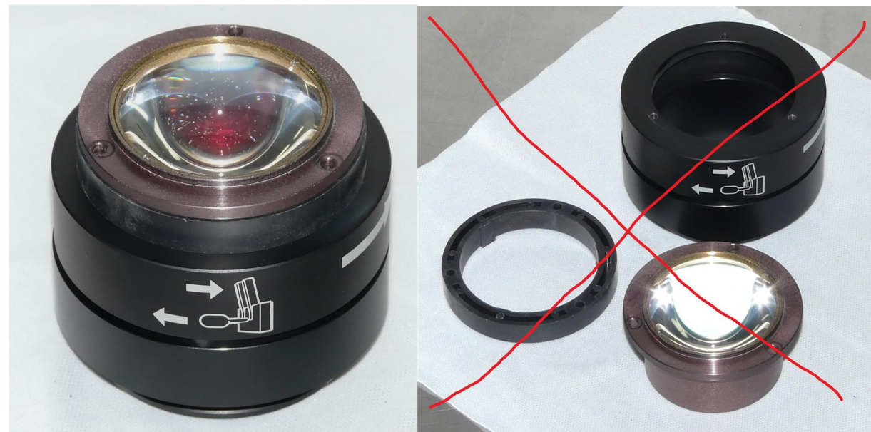
Don't let the collector lens fall out of the housing after removing the screws.
