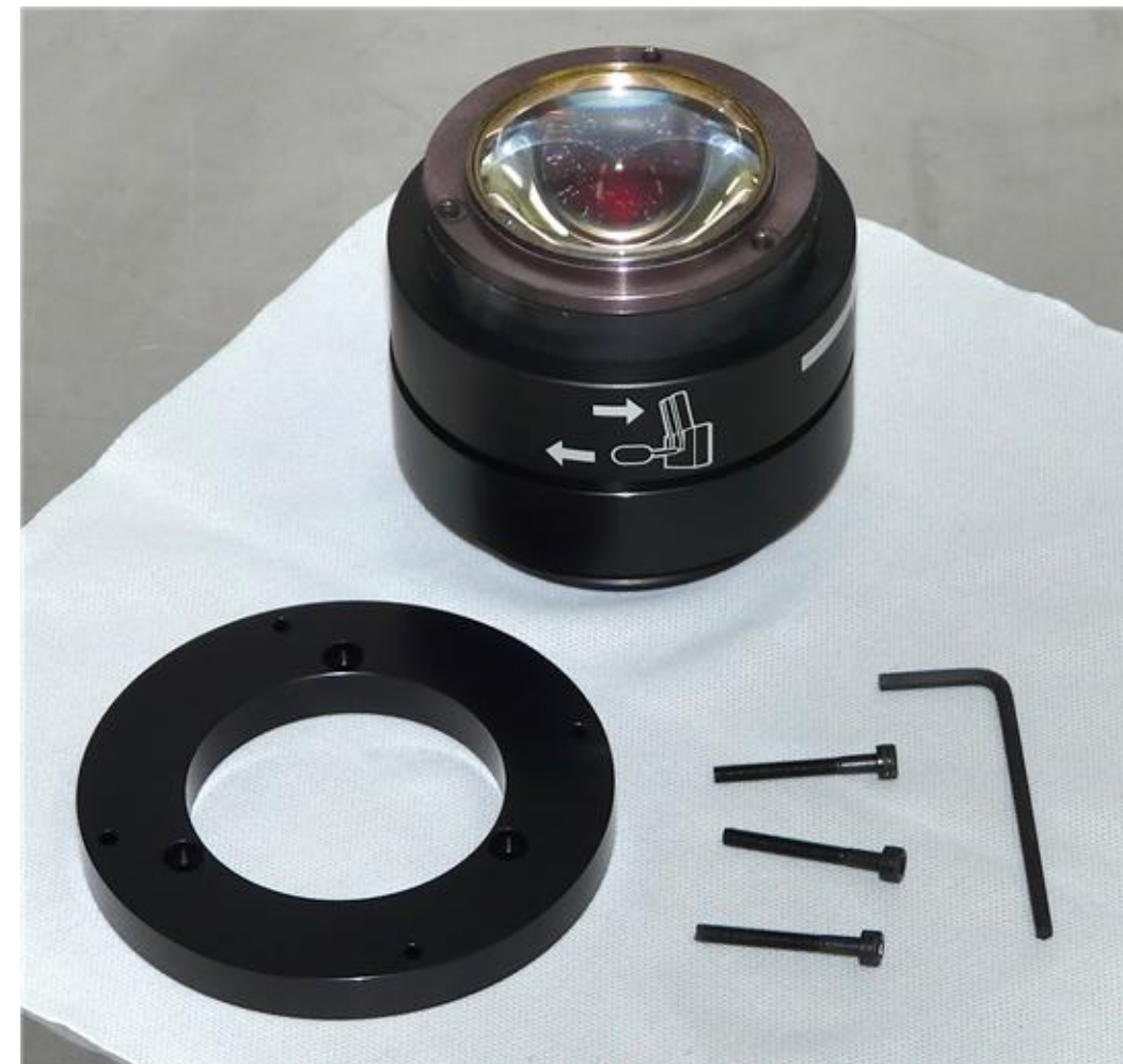
Ready to attach adapter to collector lens assembly.
