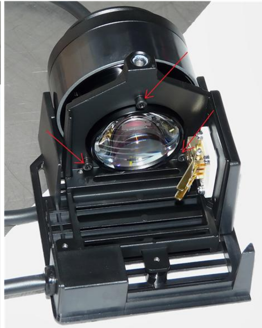
Open the lamp housing and remove the three socket head cap screws (use the 2.5mm hex key) to remove the condenser lens.
