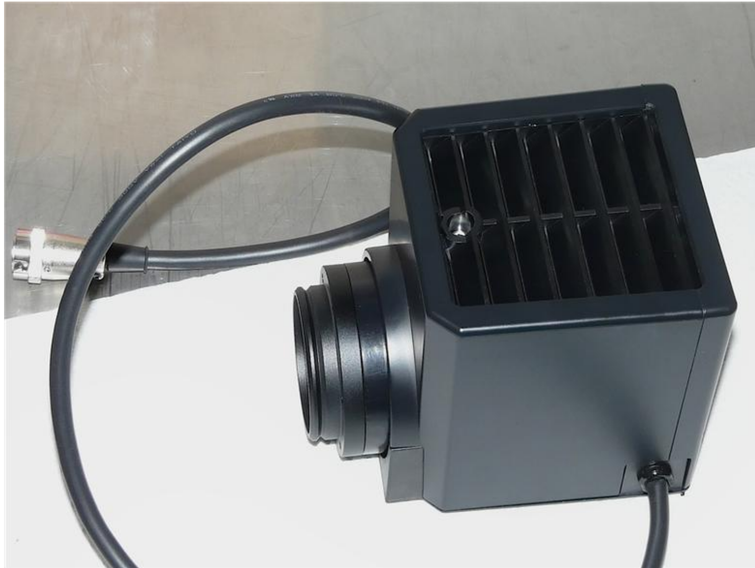
Remove the lamp housing from the microscope.
