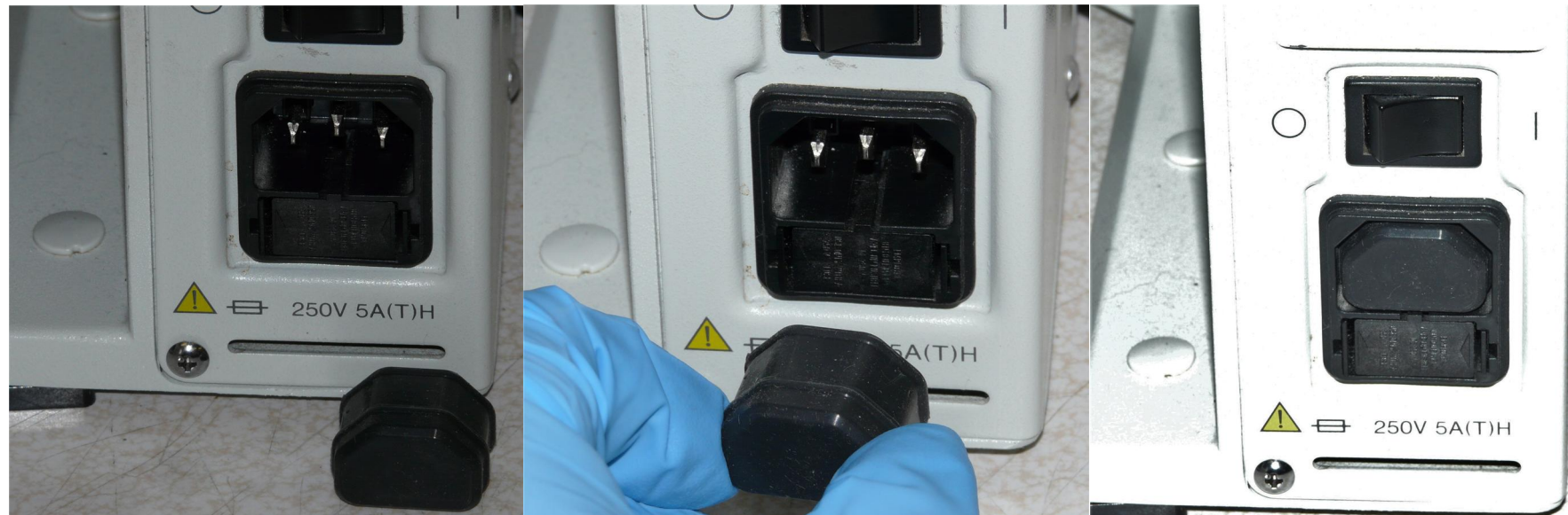
(Optional) Installation of PN 10736 rubber plug is shown above.
