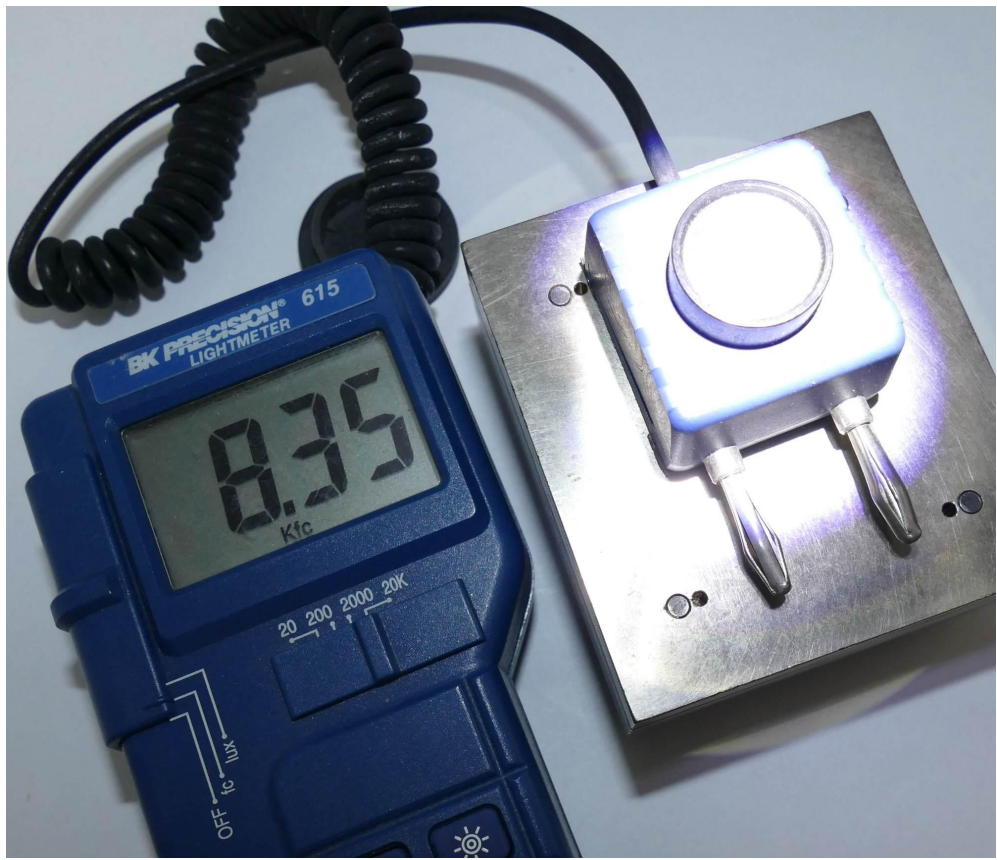
Far Left Image. Unit pushed in all the way to produce 1.9 inch wide squareish pattern with rounded corners. Near left image. Illuminator adjustment same as far left. Note 8.35Kfc light intensity - just over twice as bright. Both at 12 inches, microscope to lighted surface.
