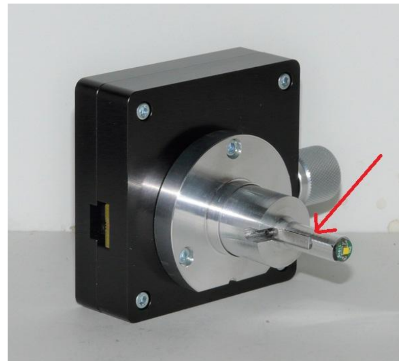
(1) Loosen the set screw on the side indicated by the red arrow. Remove the aluminum tube.
