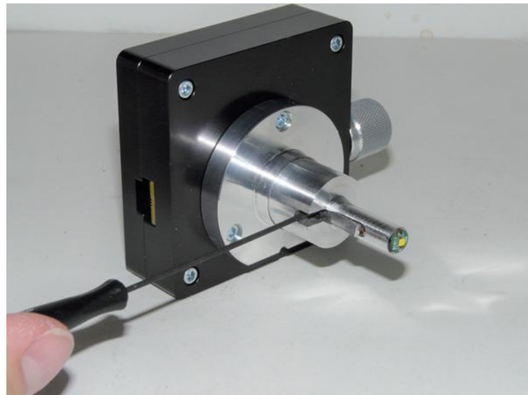
*Tighten the screw makes the clamp holds the illuminator to the fiber optic port.
