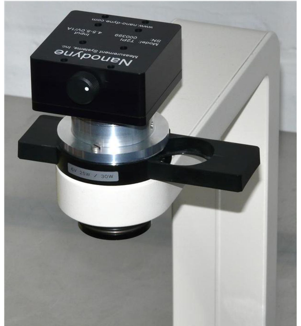
(2) Insert PN 10983 Illuminator Assembly into the adapter ring and secure in place using the 5/64 hex key to tighten the set screw. After attaching the power supply, the unit is ready to operate. To avoid confusion it might be good to black out the "6V 25W / 30W" text from the original illuminator with a permanent marker.
