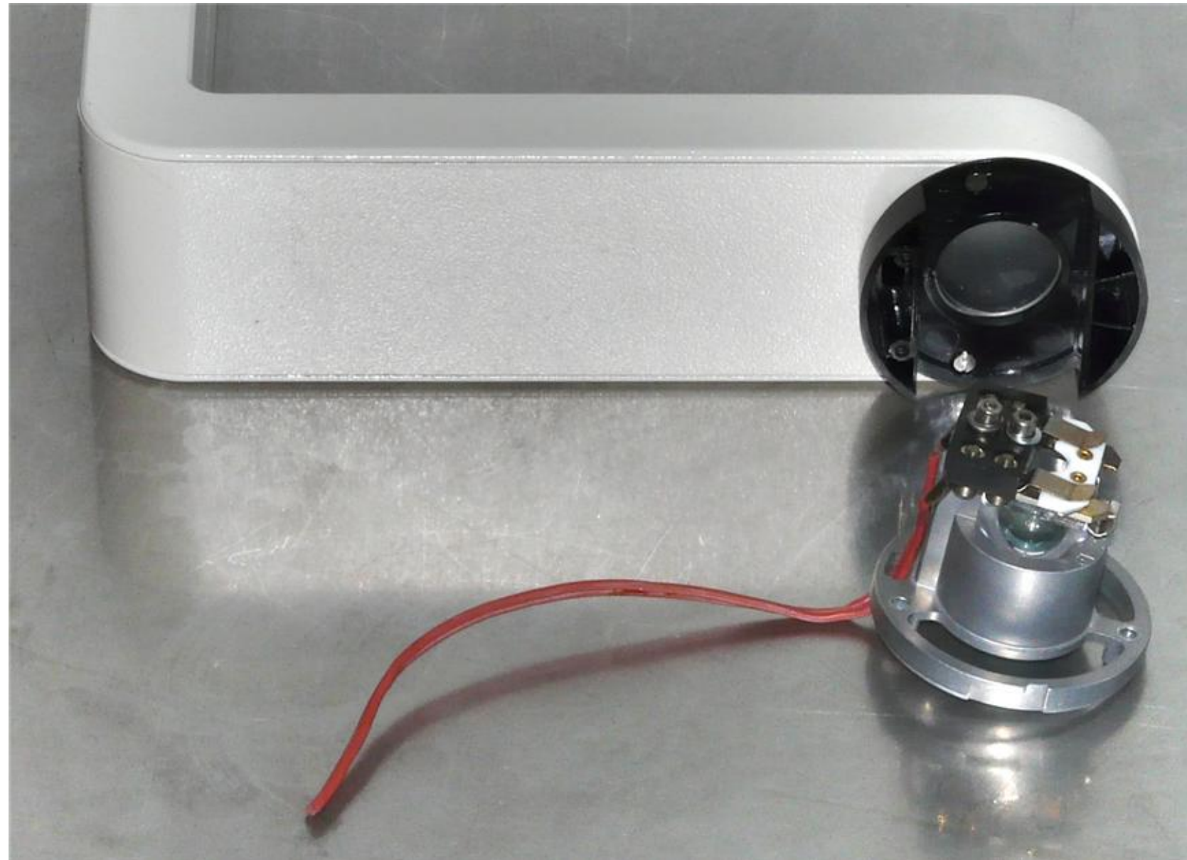
(1) Pull the illuminator assembly free from the arm as shown above. It is no longer needed.
