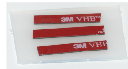
Tape to secure wires.
