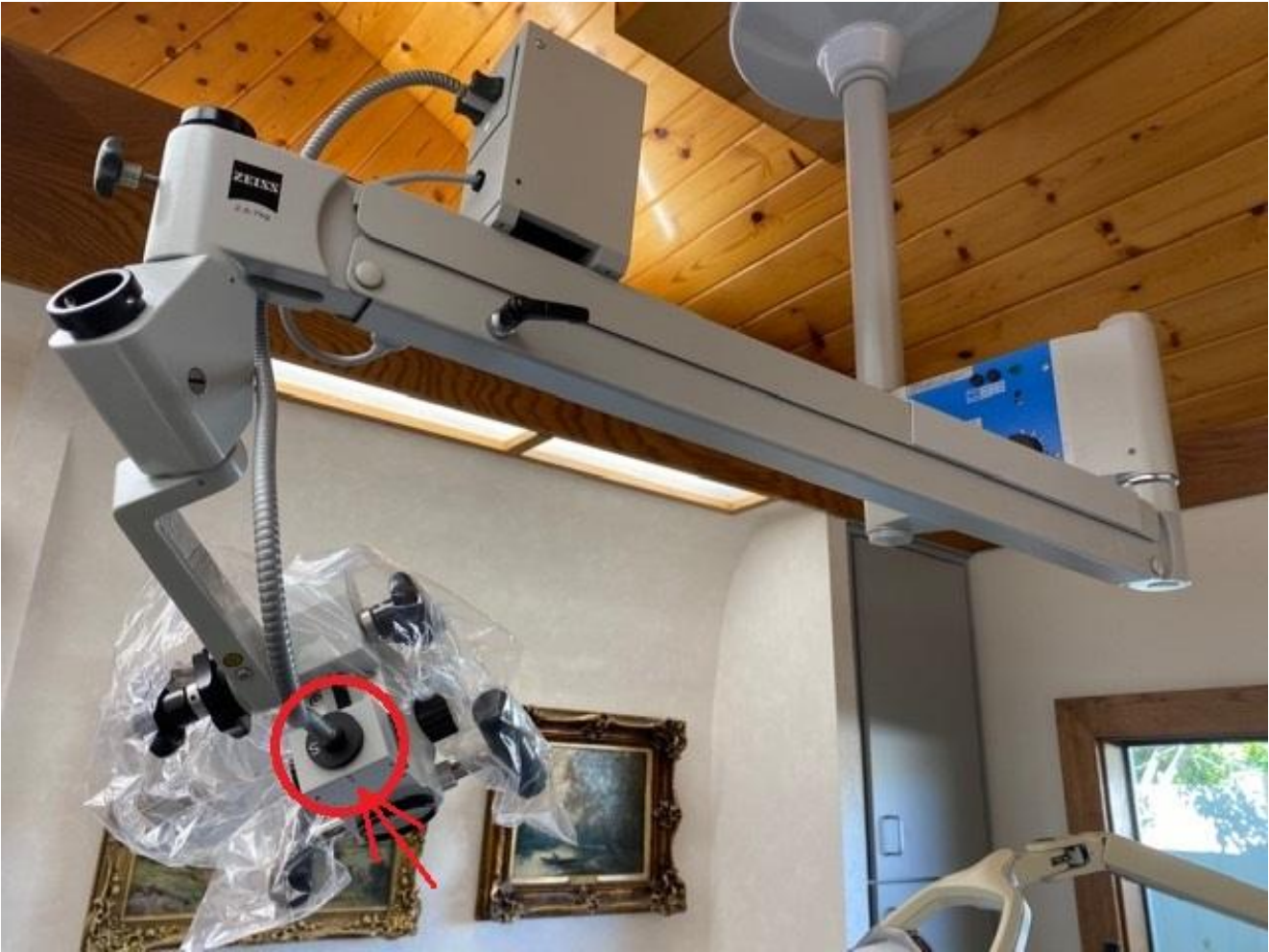
The Nanodyne illuminator replaces all of the original electronics. The fiber optic cable is eliminated also. The arrow above points to the set screw that holds the fiber optic cable in place at the microscope. The Nanodyne illuminator installs there, where the fiber optic cable is shown attached to the microscope.
