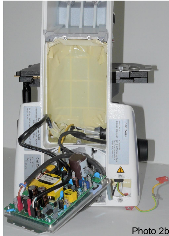
(2) Unscrew and remove the aluminum plate holding OEM PCB.
