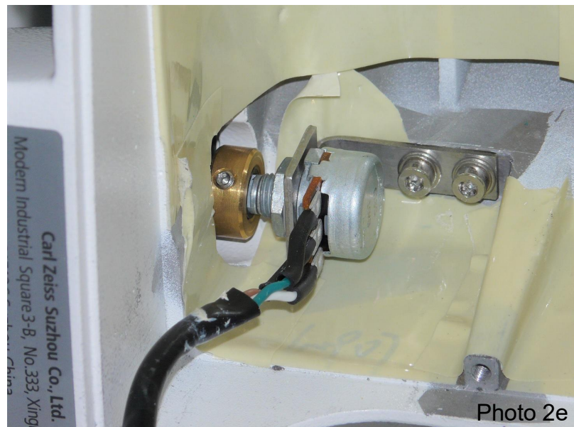
(5) Loosen the set screw on the pot knob. Remove it.
