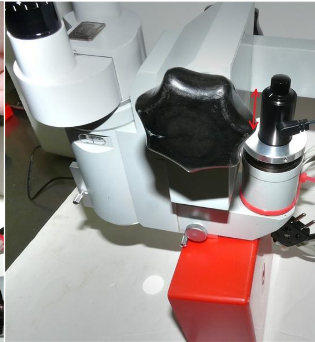
(2) Adjust the position of the illuminator up and down slightly to find the best position. Either set it to form a crisp well focused circle when the microscope is focused on that surface, or see what looks best though the eyepieces.
