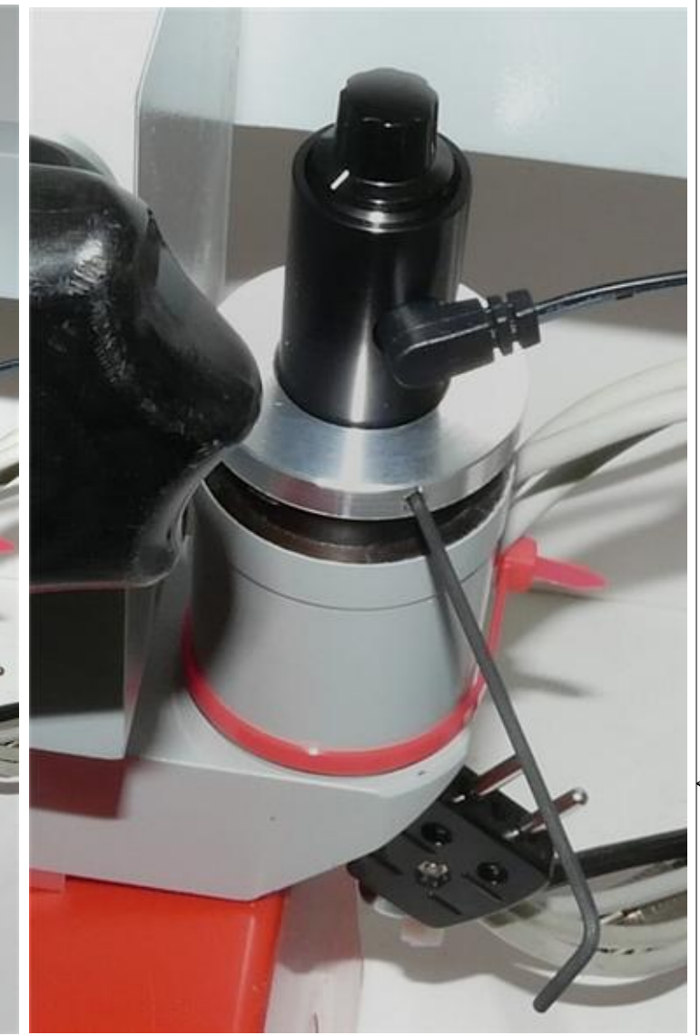
(3) Lock the illuminator into the best position with the hex key. It is now ready to operate.
