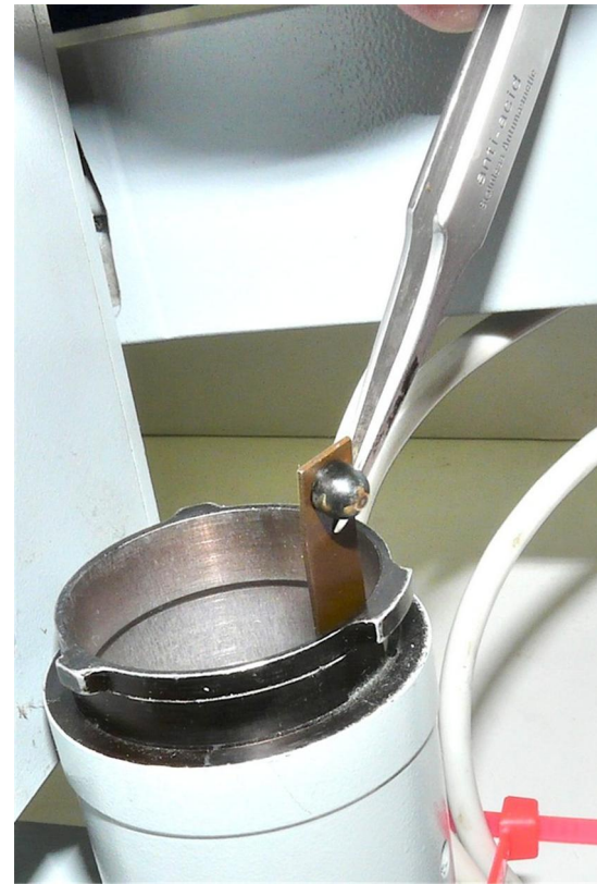
(6) Remove the spring/ball latch.
