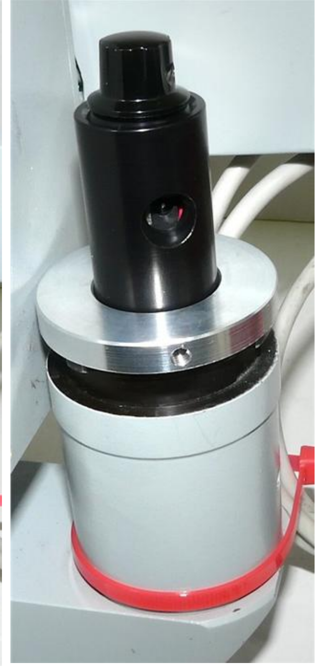
(4) Nanodyne illuminator fully inserted.
