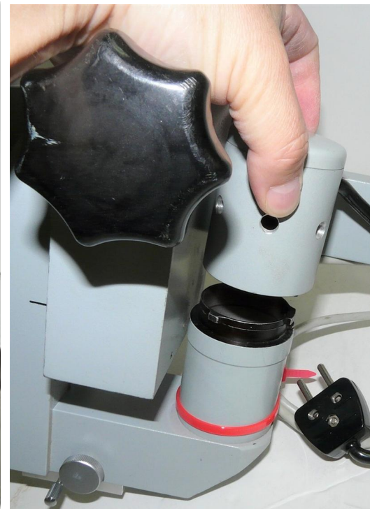
(2) Twist and remove cover.
