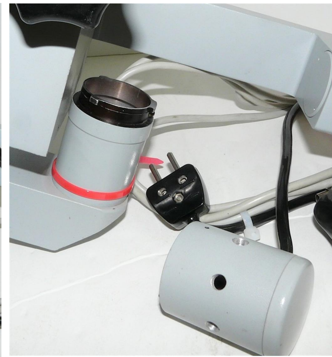
(3) Lamphouse cover removed.
