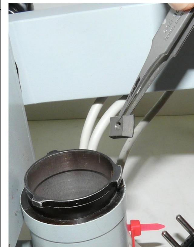
(5) Remove the nut the screw was in.
