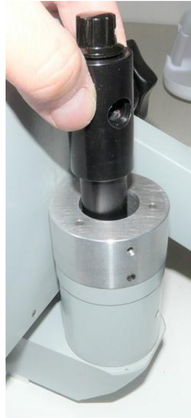
(3) Insert the Nanodyne illuminator into the adapter.
