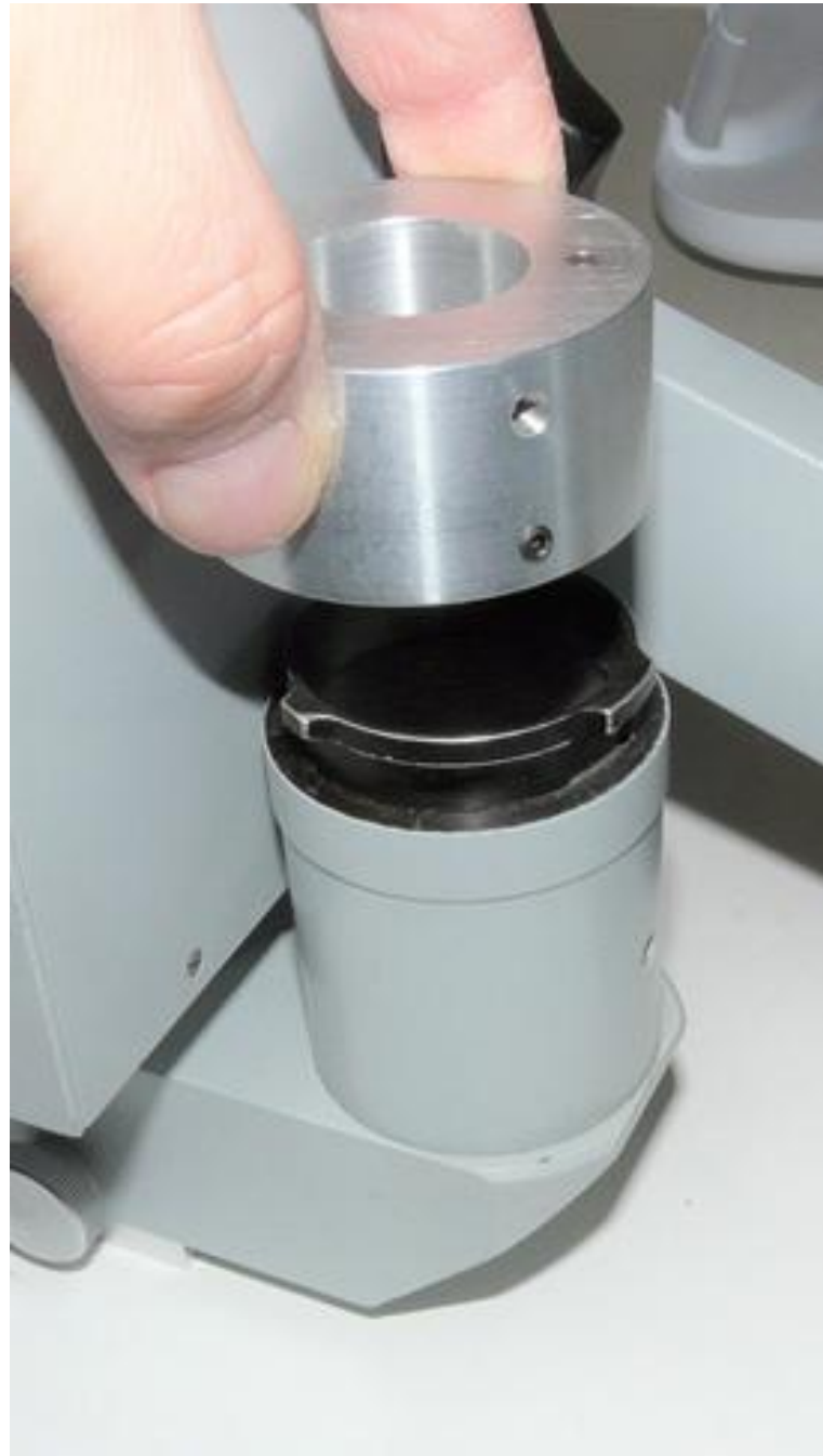
(1) Insert the Nanodyne adapter into the lamp housing.
