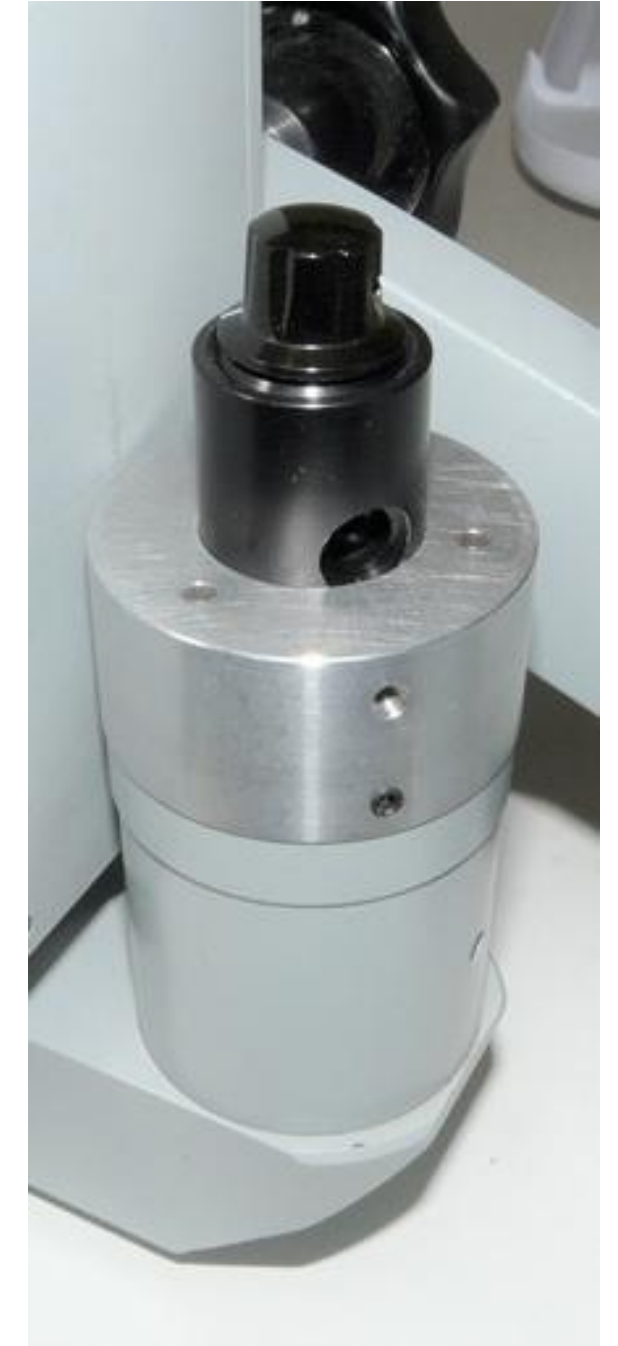
(4) Nanodyne illuminator fully inserted.
