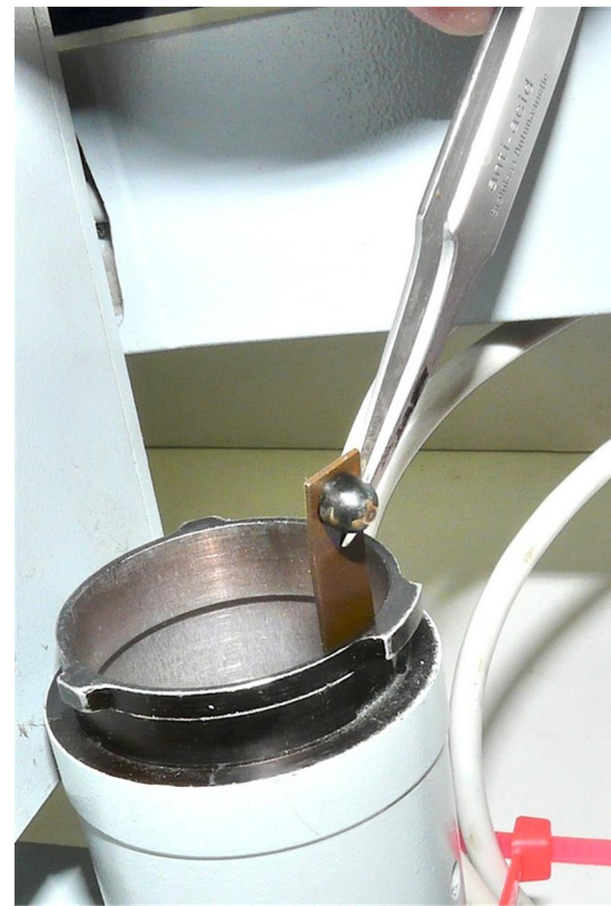
(6) Remove the spring/ball latch.
