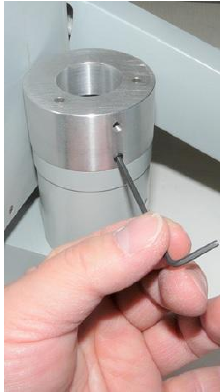
(2) Tighten set screw to install Nanodyne adapter over the lamp housing using a hex key provided.
