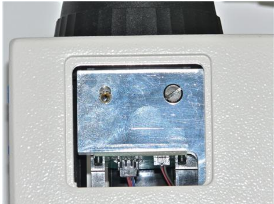
(2) Nanodyne illuminator Assy partially attached.
