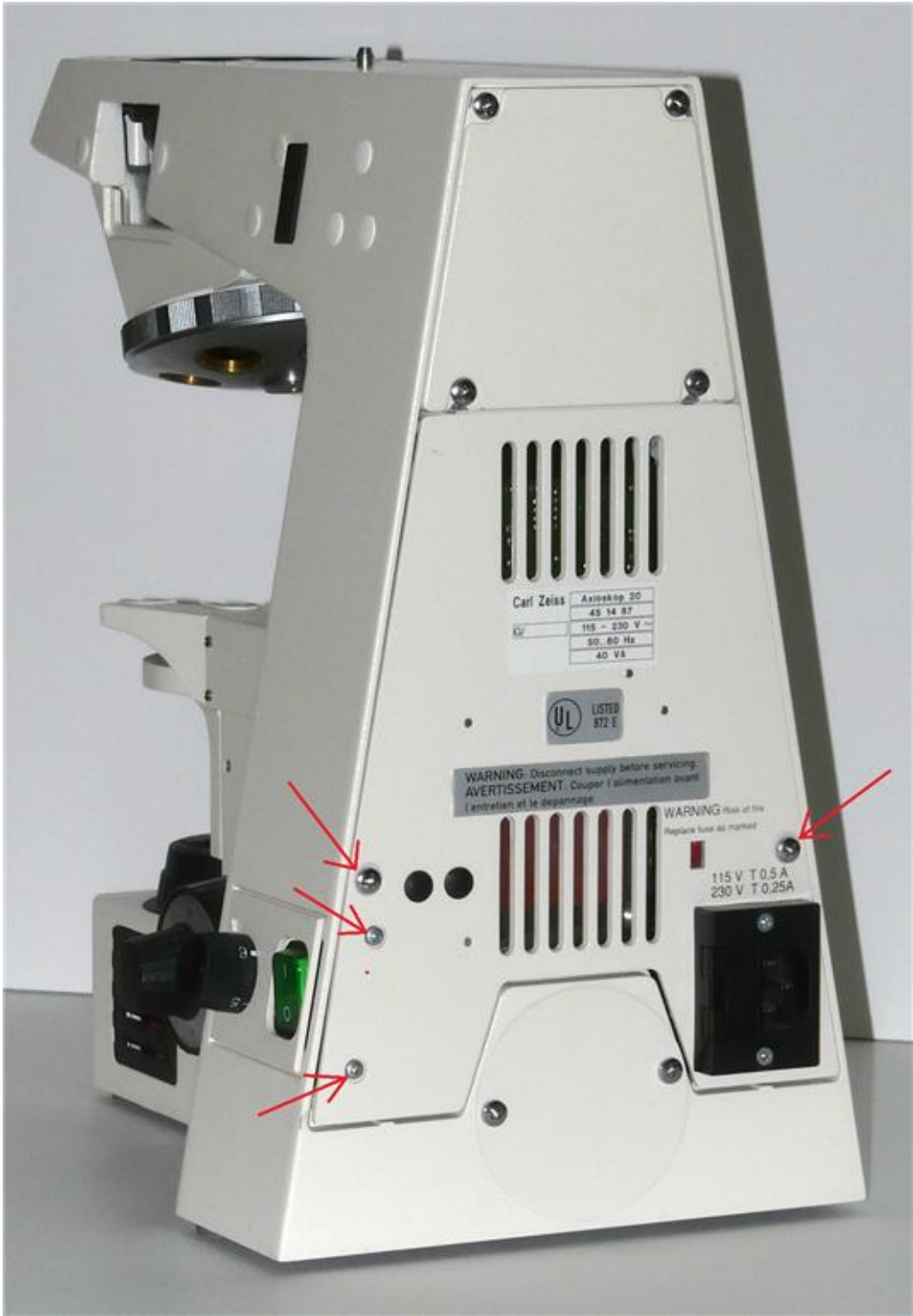
(1) Remove the 4 screws indicated above.
