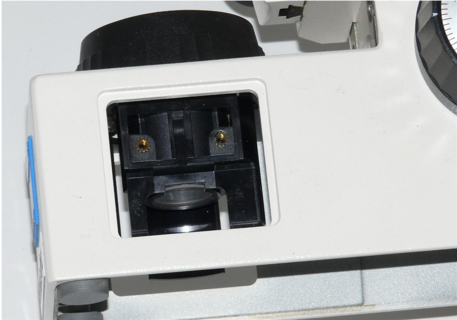
(1) The Nanodyne illuminator will be mounted just like the old halogen lamp assembly, using the same screws.
