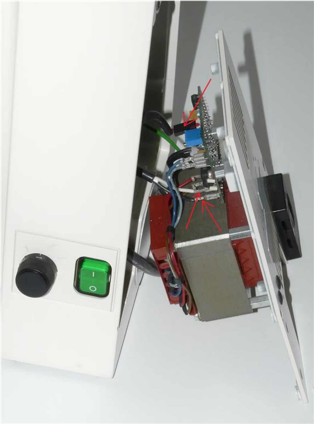
(3) Pull the black connector off of the circuit board. Pull the white and black wires off the transformer. If these wires are too tight to pull by hand use a pliers (see next sheet).
