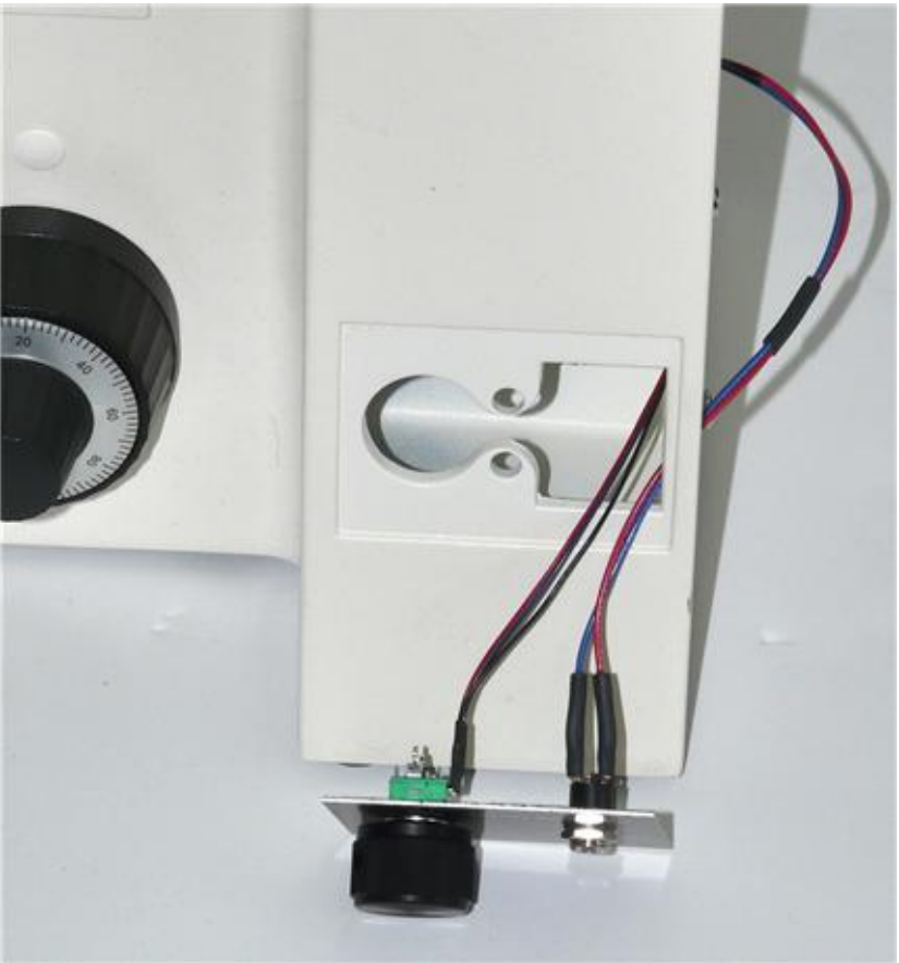
(2) Route the cables through the side panel hole in the microscope as shown above.
