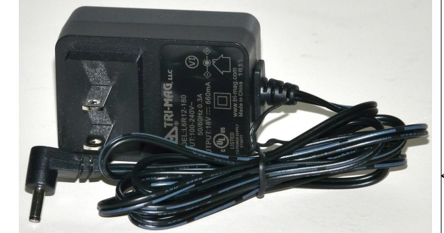
PN 11700 Power Supply - Tri-Mag 18V 660mA Fixed Blade US Input 1.35mm ID x 3.5mm OD RA plug output, 6 foot.
