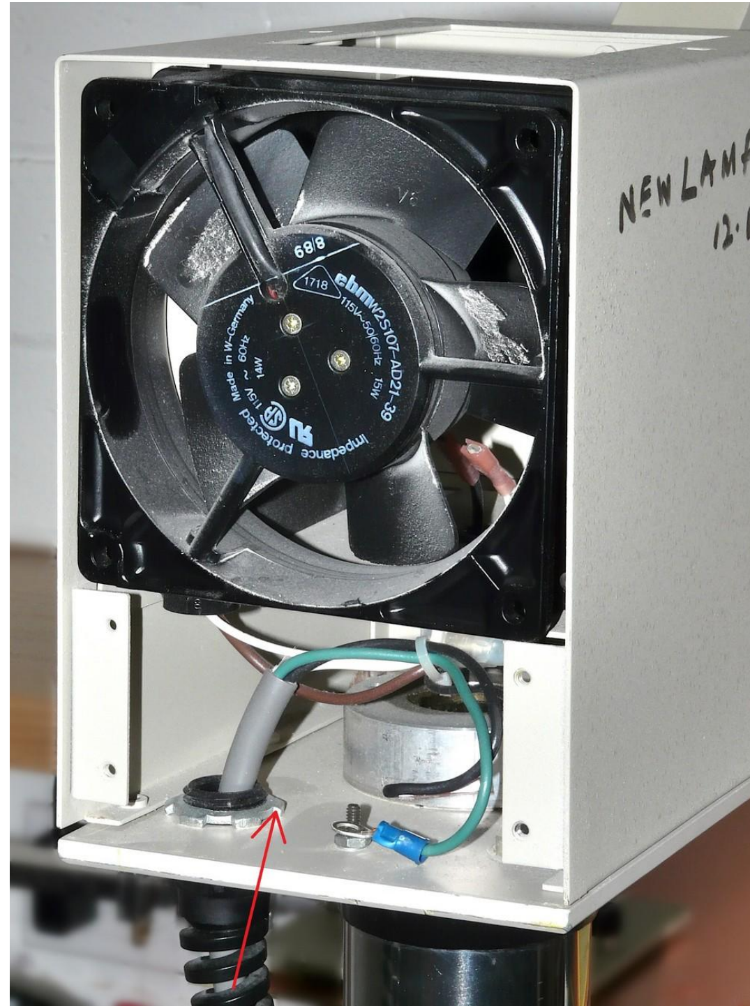
(2) Remove back plate. Disconnect or cut wires, remove nut (see red arrow) to free AC power cord. Then replace back cover.
