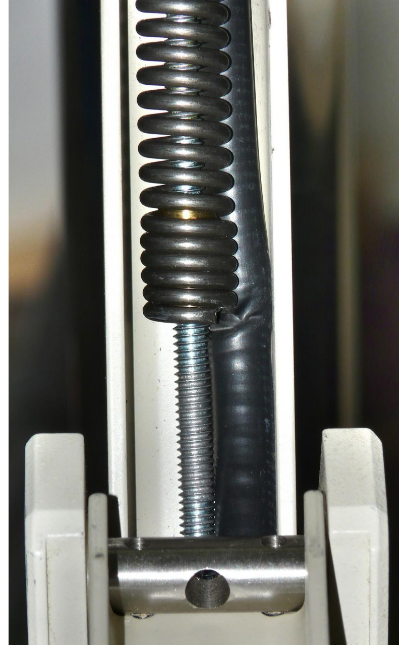
(5) The OEM set up has the fiber cable pinched between the arm and the tension spring. You can remove the screw in the tension spring (see photo 13) to make it easy to remove the fiber cable, but you might get carpal tunnel before you are done. We suggest just using brute force to pull the cable out. You might damage the cable, but it won't be needed anymore.
