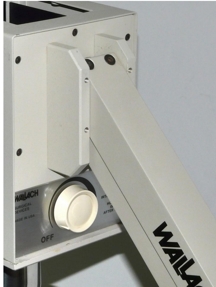
(2) Replace the 2 screws in the articulating arm. Manipulate the angle of the short arm if needed to line up the holes.
