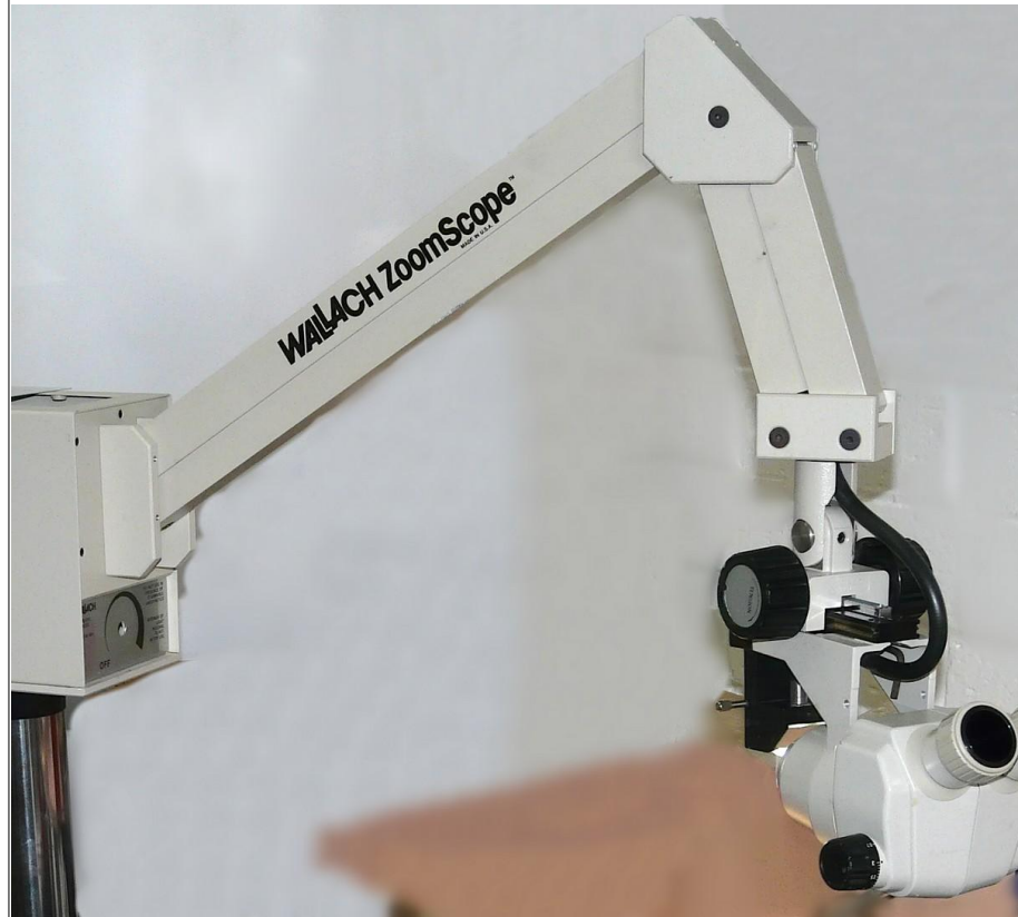
(1) The fiber optic cable runs from the lamp at the far left to the microscope at the far right, through the articulated arm.
