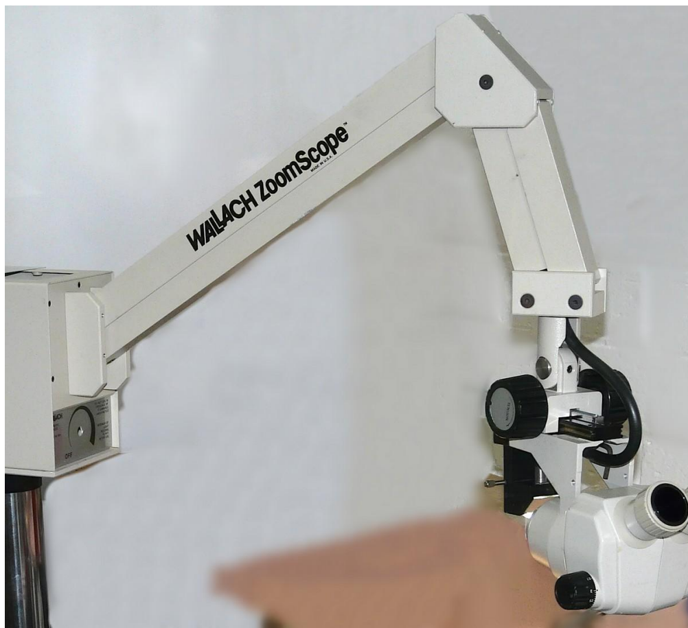
Original system. Fiber optic cable brings light from 50W Halogen bulb (at left side) through articulating arm to microscope. (OEM adjustment knob and lamp cover are missing in the photo)
