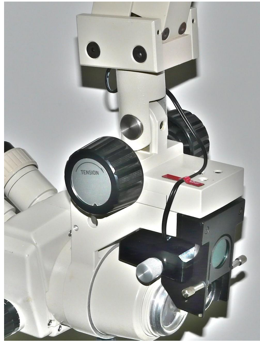
(1) Connect the power cord to the illuminator, and route it as shown so it will not bind as the microscope is rotated.
