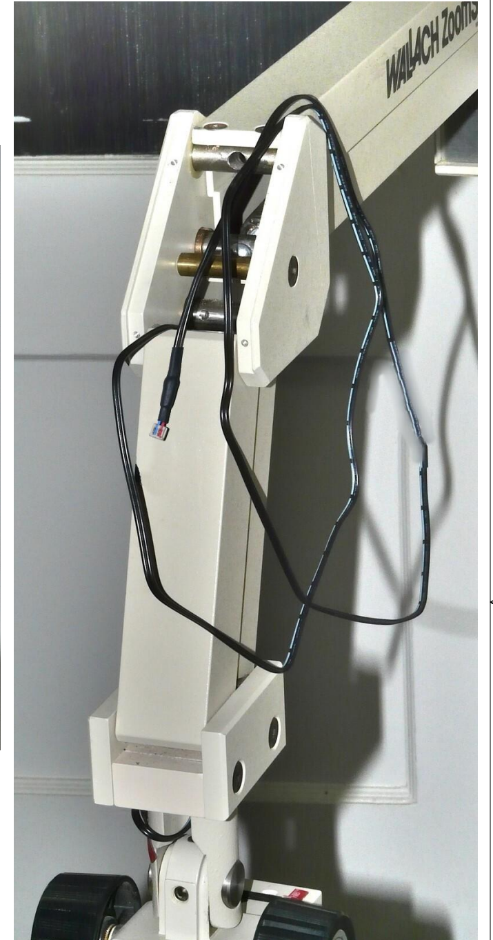
(2) Route the power cable up through the short portion of the articulating arm as shown.
