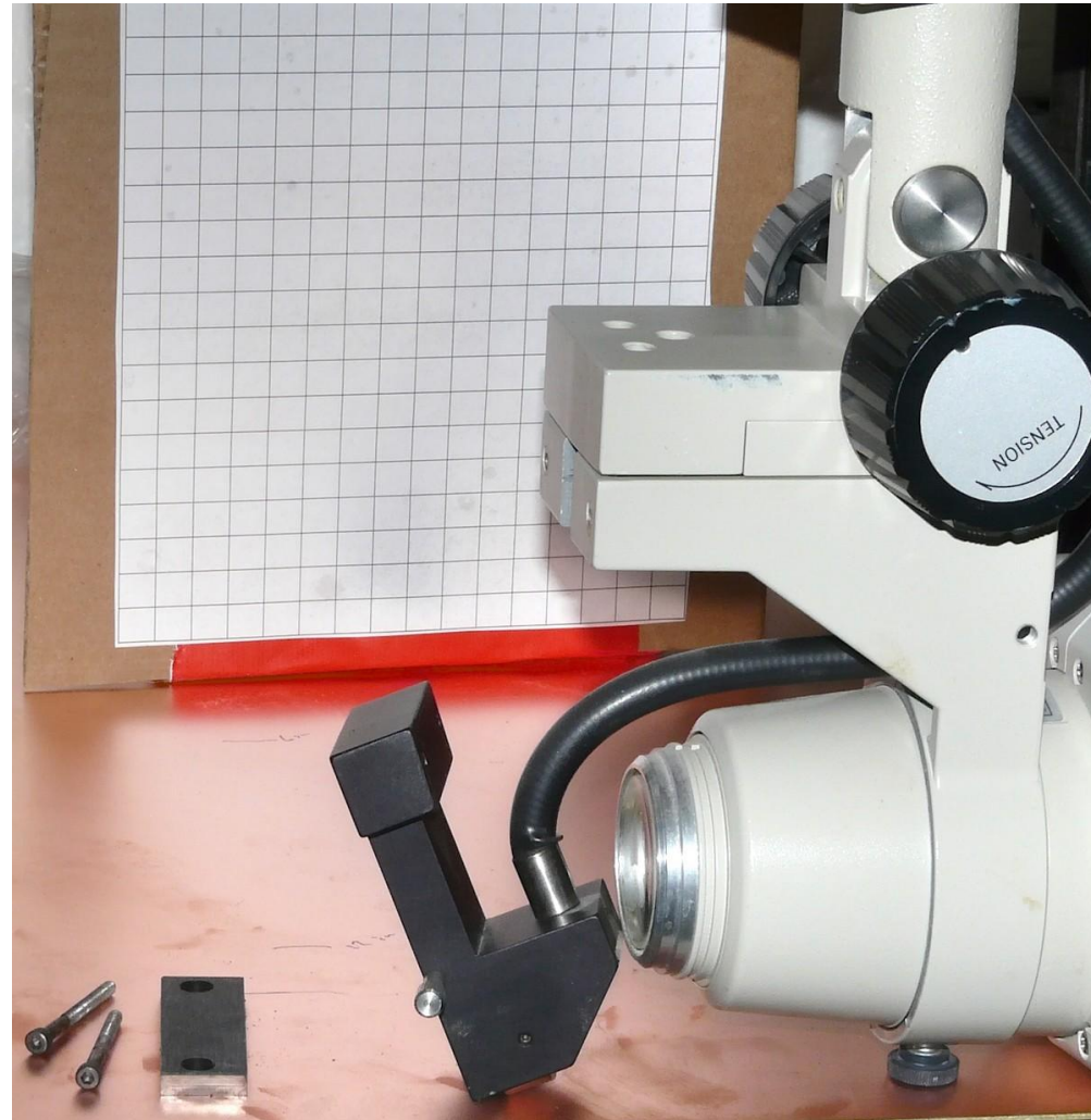
(3) Free the OEM lens/mirror/fiber cable assembly by removing the two 6-32 screws using the 7/64 inch hex key. Everything but the fiber cable will be re-used.
