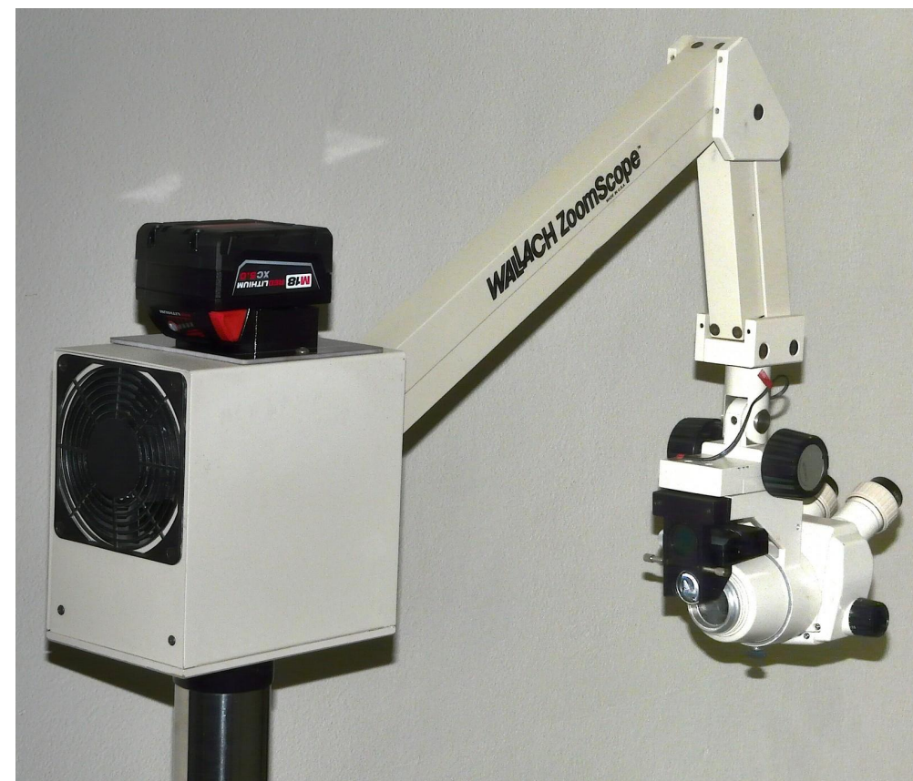
Nanodyne illuminator installed on microscope. Battery pack (optional add-on with additional cost) on top of original lamp housing provides for cordless operation. AC to DC power supply also included for operation without the battery.
