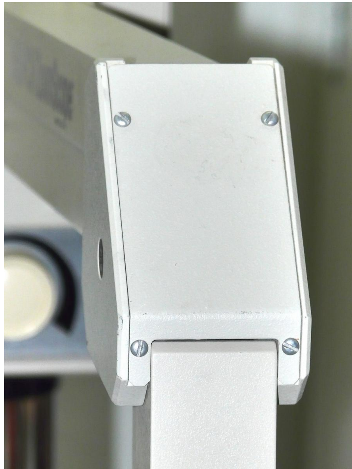
(1) Remove the cover on the elbow of the articulating arm. It is held by the 4 screws.
