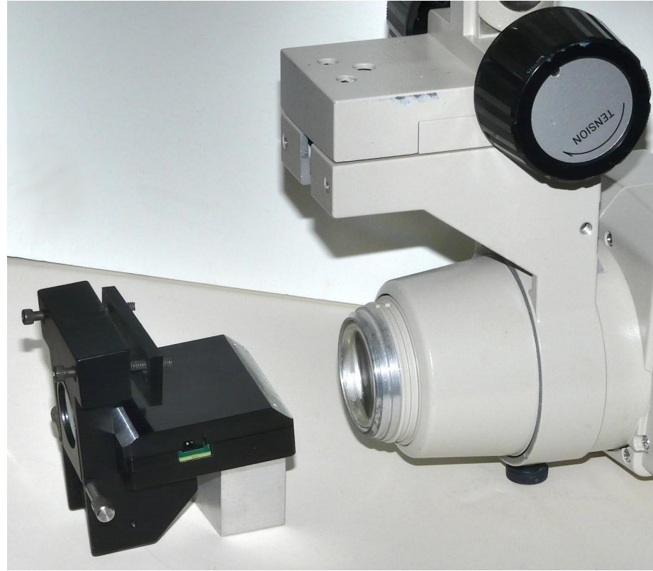
(1) New illuminator assembly ready to attach to microscope (block under illuminator is just support for photo).
