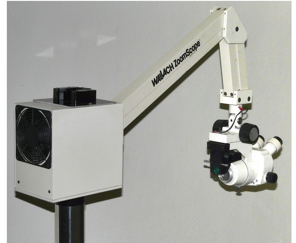
(3) Turn the power module right side up and secure to the lamp house with the two 10-32 button head screws. Use the 1/8 inch hex key to tighten.
