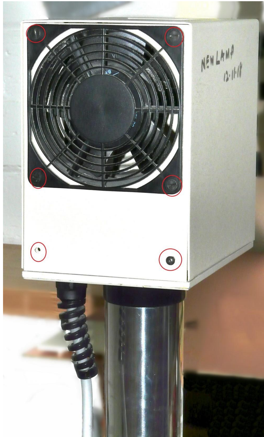
(1) Remove 6 screws from back plate.
