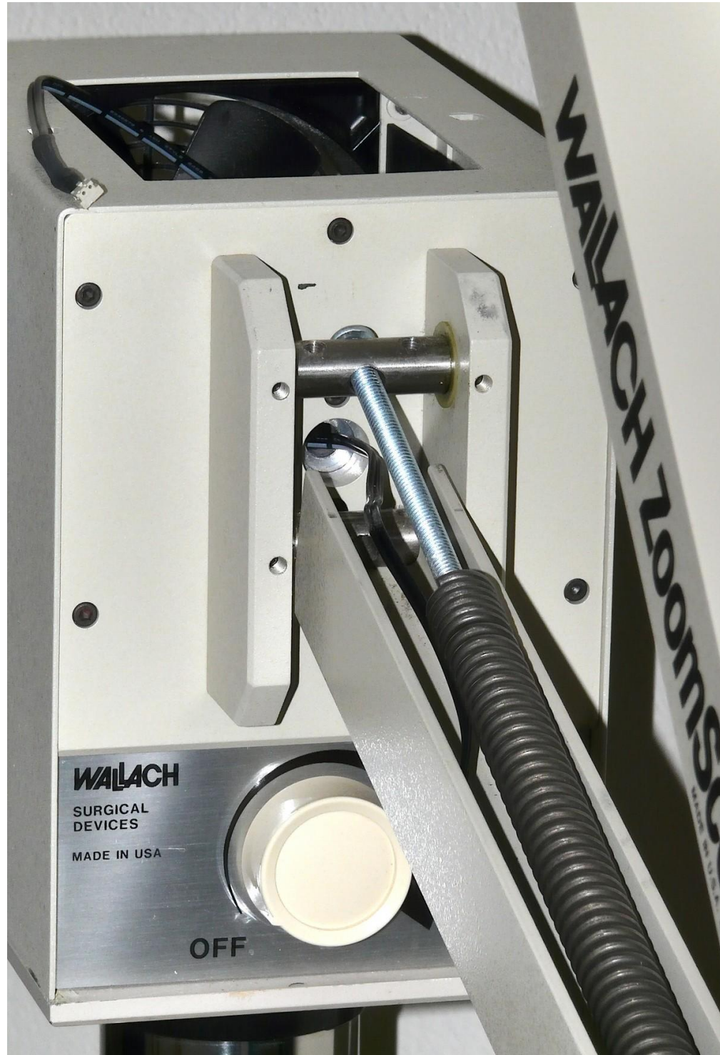
(1) Route the power cable up the long articulated arm, and feed it through the hole for the fiber optic cable, into the lamp housing.
