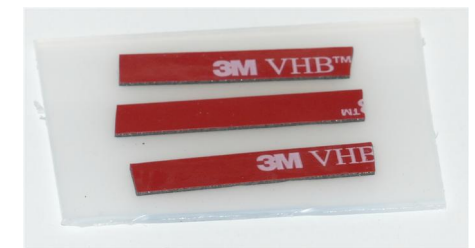
Tape to secure wires.
