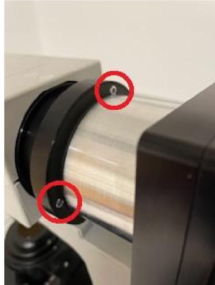
(2) Tighten the original 3 screws (red circle) using 2.5mm hex key provided.
