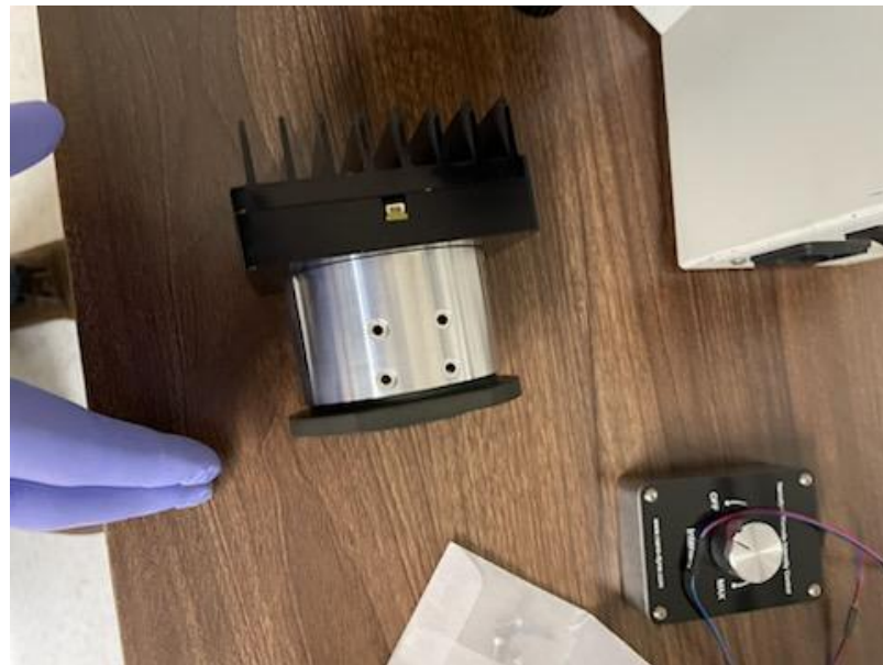
(5) Fully insert the OEM collector lens assembly to the Nanodyne illuminator.
