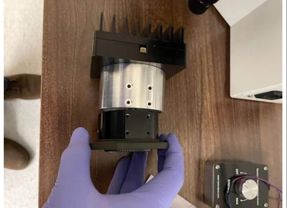
(3) Attach the OEM collector lens assembly to the Nanodyne illuminator.
