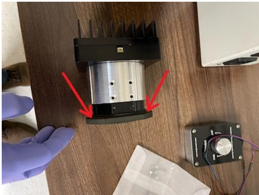
(4) Place the original 3 screws to the lens assembly before fully insert the Nanodyne illuminator.
