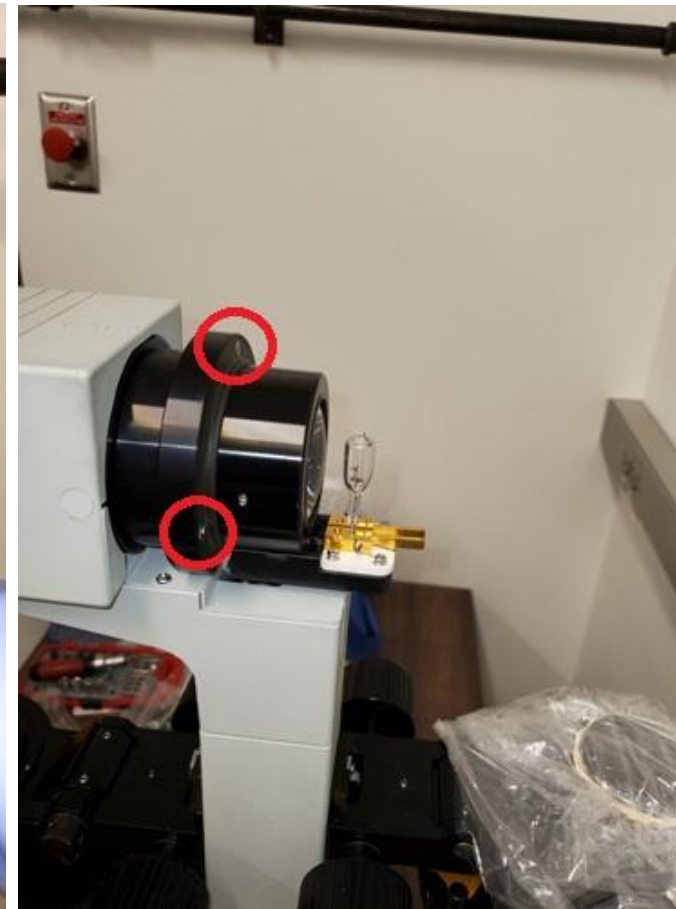
(3) Remove the 3 screws (red circle) holding the collector lens assembly. Use the 2.5mm hex key provided. Keep the original screws for the later installation.
