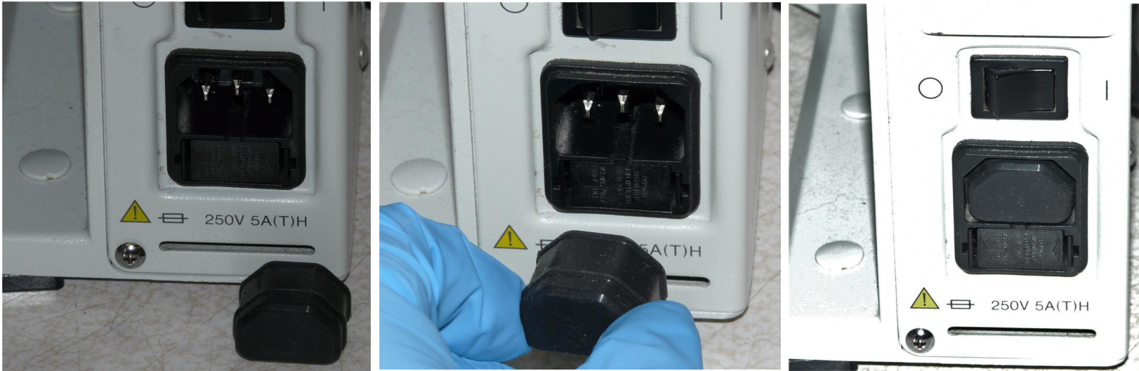
(1) Installing PN 10736 rubber plug in AC receptacle to deter connection of obsolete AC power.
