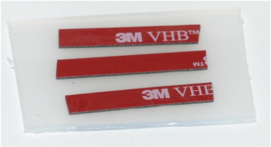
3M VHB tape to secure pot cable
