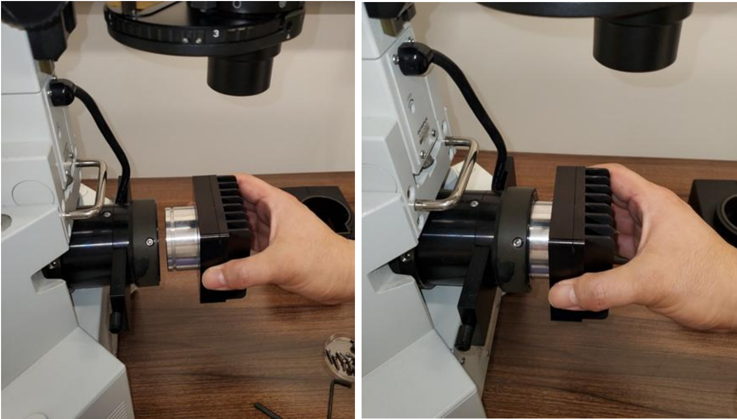
(2) Insert the illuminator into the microscope port and secure it the same way as the original. Keep it pressed firmly in place until the microscope screw has secured it, to ensure good alignment.
