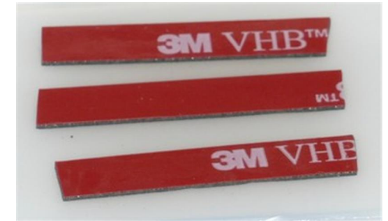
Tape to secure wires.
