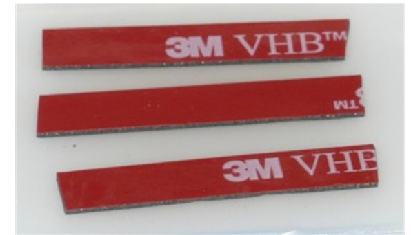
3M VHB Tape to secure wires.
