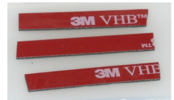
Tape to secure wires.
