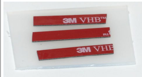
Tape to secure wires.
