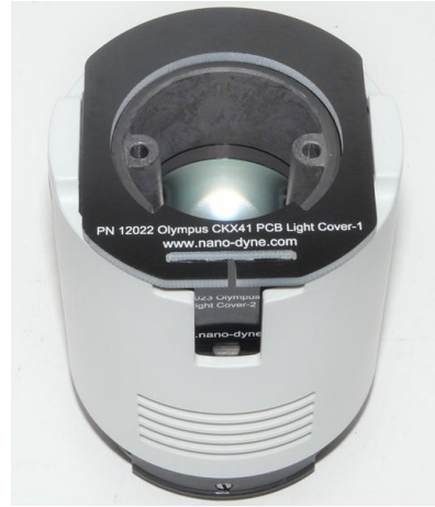
PCB light cover installed.
