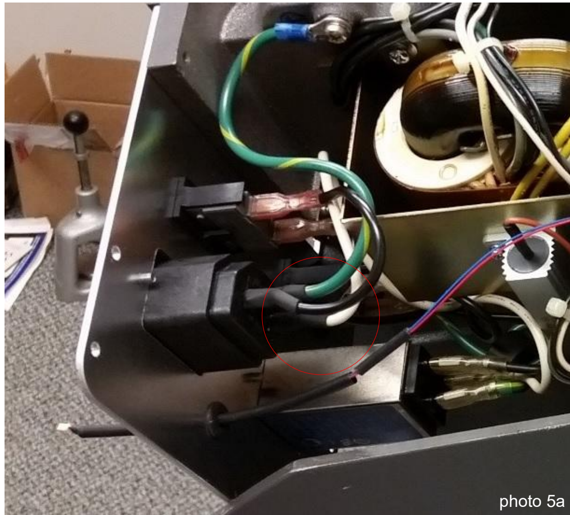
Install PN 10736 rubber blocking plug to deter connection of unneeded AC power.
