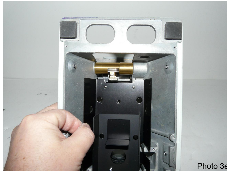
Unscrew and remove the black metal cover.
