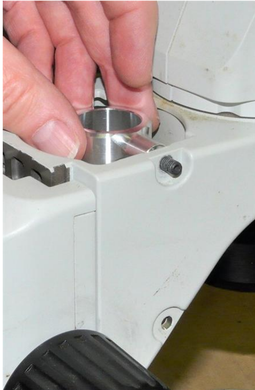
(1) Place the adapter in the microscope as shown.
