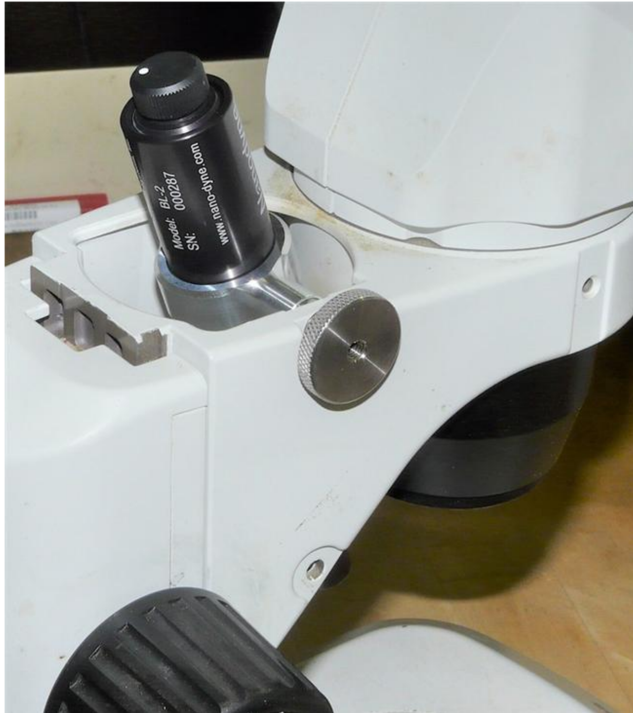
(1) Place the illuminator in the adapter. A small force will seat it securely.
