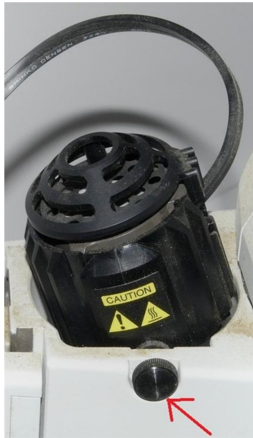
(2) Remove the thumb screw to remove the illuminator.
