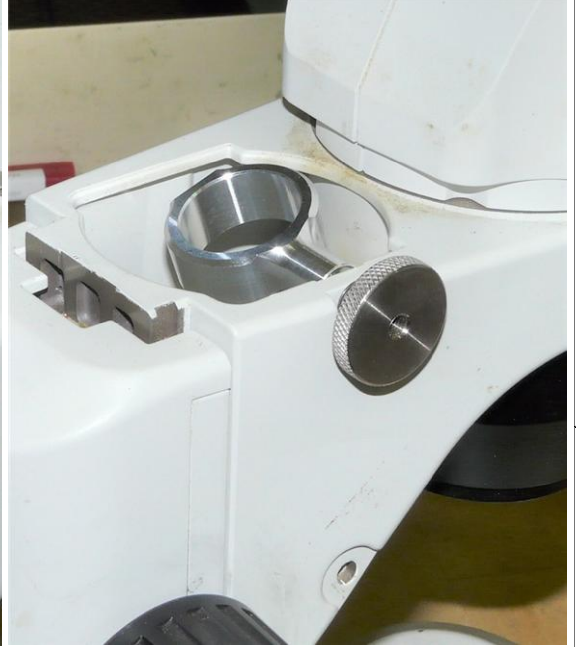
(3) Screw the thumb nut onto the threaded stud.
