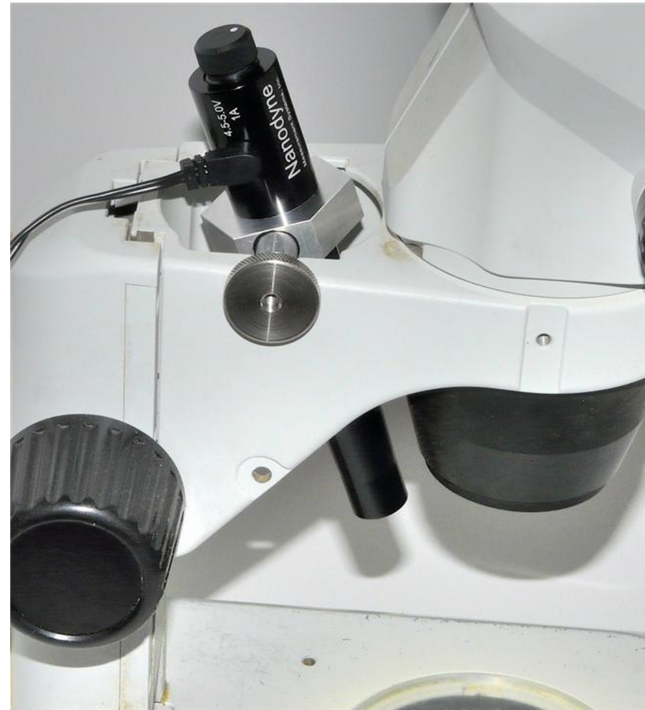
(2) Plug the power cord into the illuminator as shown. Plug the other (USB) end into the power supply. Plug the power supply into an AC outlet and the unit is ready to use. Brightness is controlled by the knob at the top. It is fully off when turned counter clockwise. There is no click off. Do not force it.
