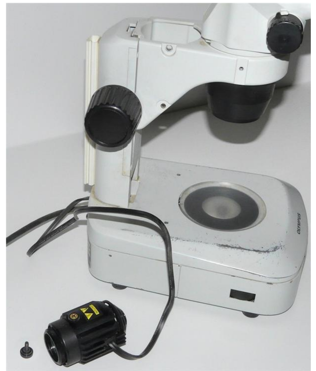
(3) The illuminator has been removed.
