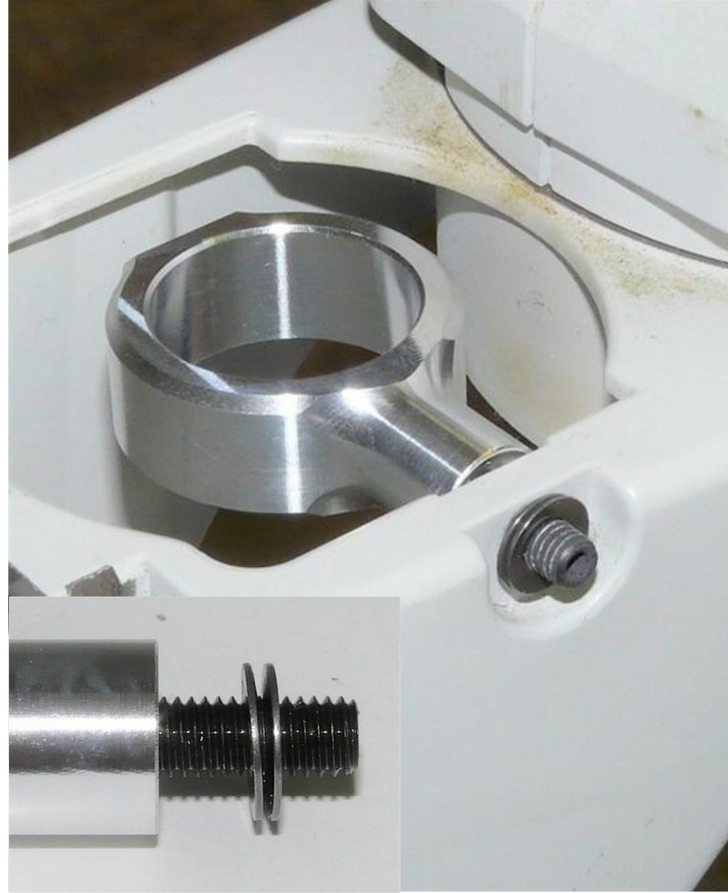
(2) Place the two bellville springs as shown.
