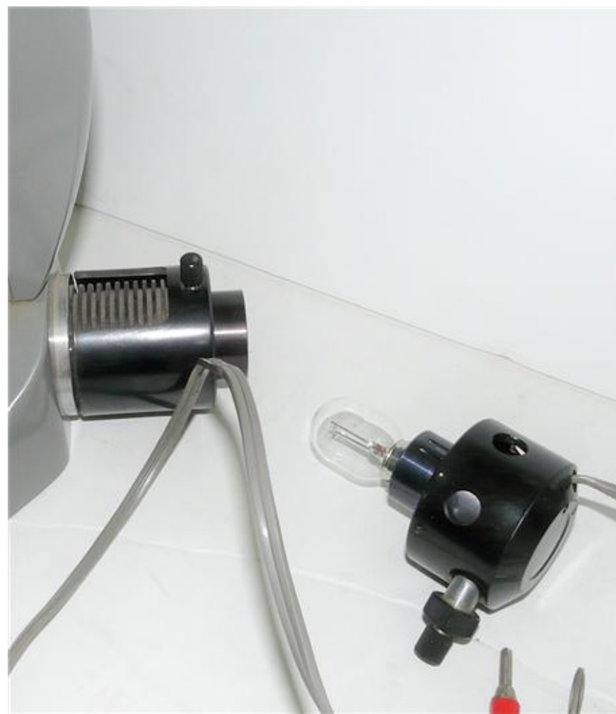
(2) Pull out the OEM lamp. It is just held in by friction.
