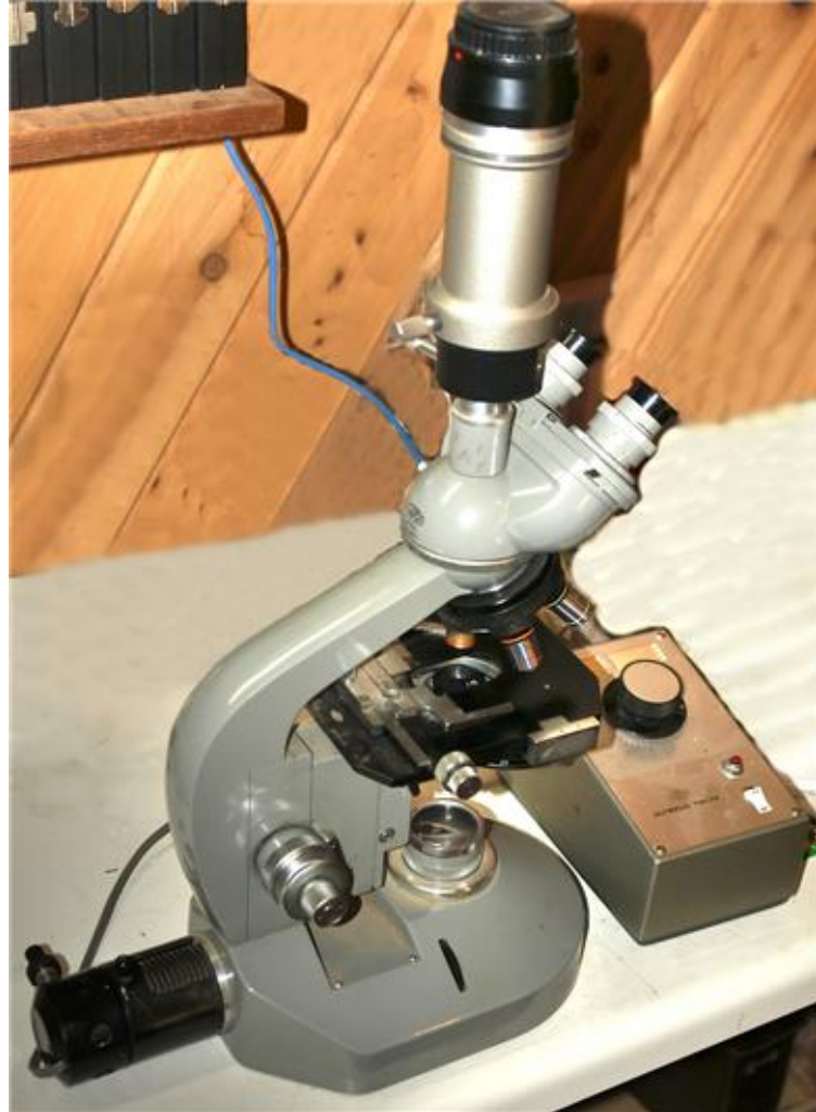
(1) Microscope with OEM lamp and power supply.
