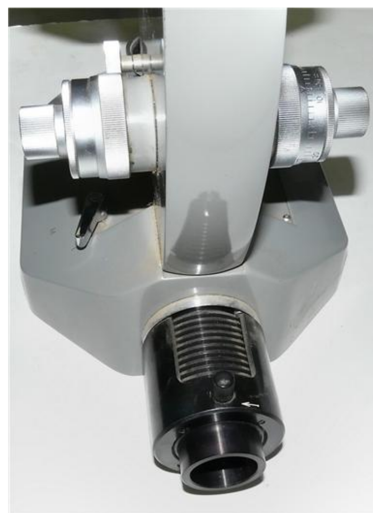
(3) Lamp removed. Note that the inner portion of the lamp mount can move in and out when the thumb screw is loosened.
