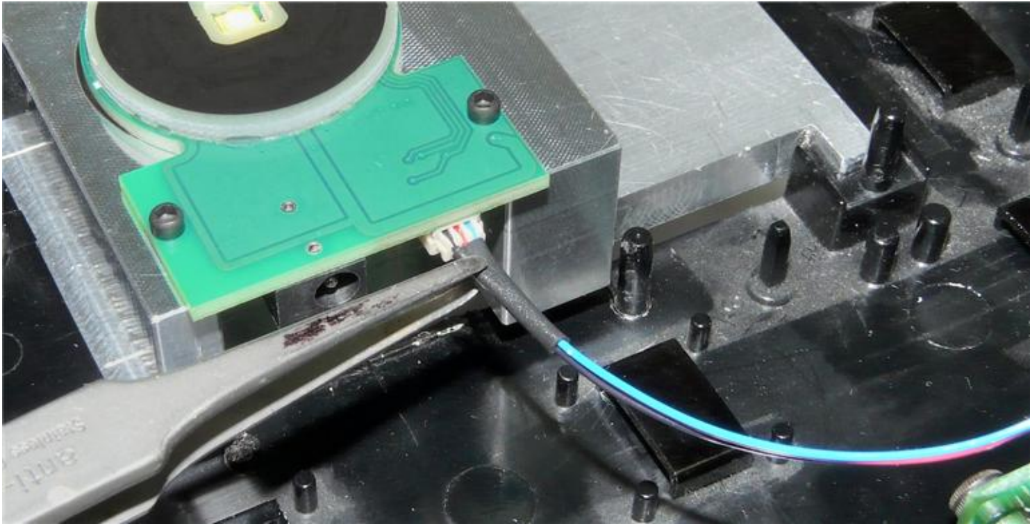
(1) Connect the pot cable to the connector under the circuit board as shown. It must be oriented as shown. It can be inserted as far as shown by holding the wires.
