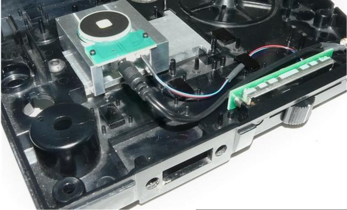
(4) Connect the power cable to the illuminator as shown above.
