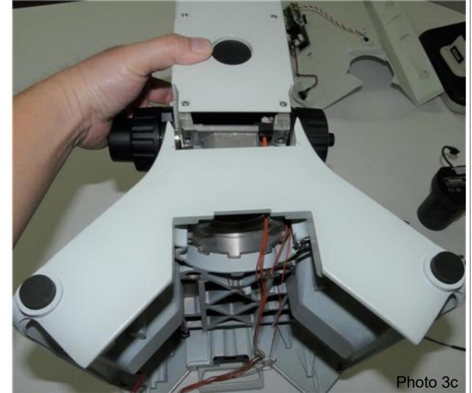
Pull out original pot cable from the existing cable ties (red circles). Unscrew using 4mm hex key and pull out the base unit as shown above.
