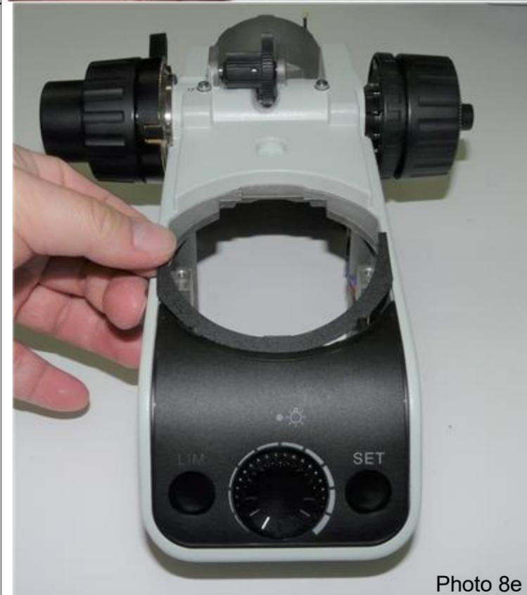
Re-install front panel and secure the cables as shown above with the existing tie wraps, to keep the cables out of the moving parts of the microscope, and the optical path from the illuminator. Insert black rubber guide (red circle) to the right place and attach the original taped cover from the base unit as shown in left.
