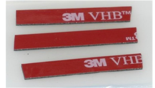
3M VHB Tape to secure wires.
