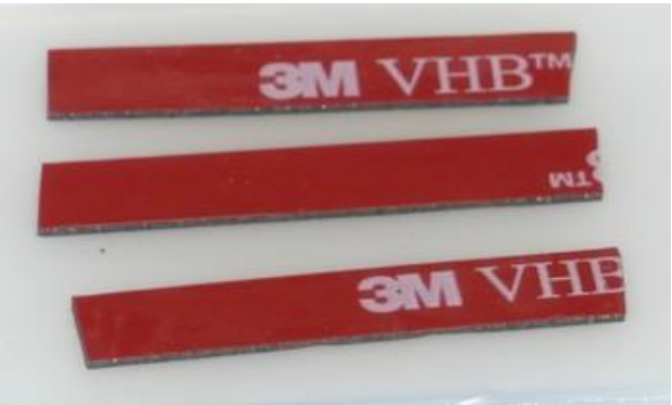
3M VHB Tape to secure wires.
