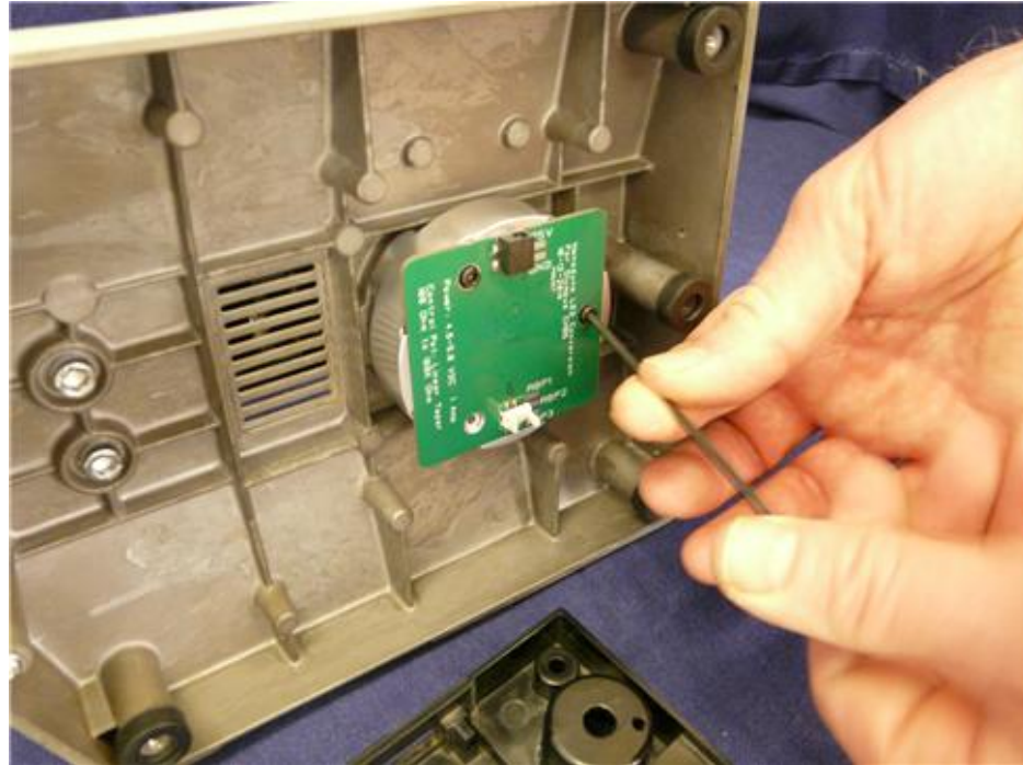
(1) Tighten the three screws with the 2mm hex key. Note that the illuminator shown is an older version.
