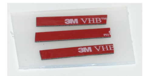
Tape to secure wires.
