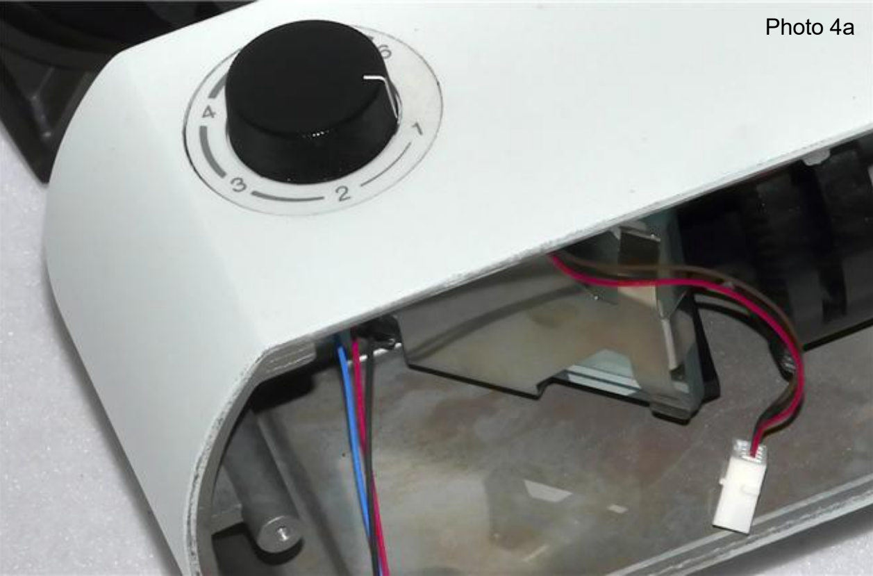
Re-install the knob on the pot with the 1.5mm hex key.
