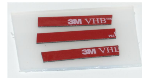
Tape to secure wires.
