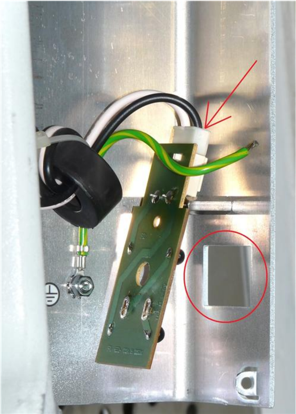
(1) Inside view of obsolete AC power input for BX51-61. (The AC input receptacle which would be mounted in the empty circled hole had been removed before we received the microscope) Remove AC power lead connection by disconnecting the socket indicated by the arrow above.
