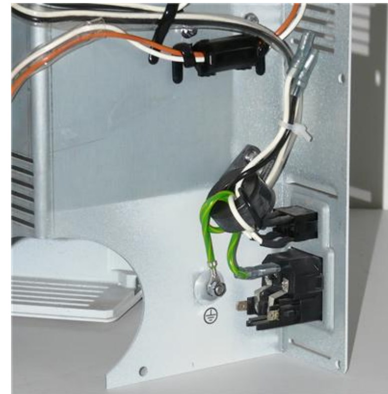
(4) Disconnect the white and black AC power leads by pulling them off of the terminals. Secure the leads as shown so there is no way they can contact the terminals.
