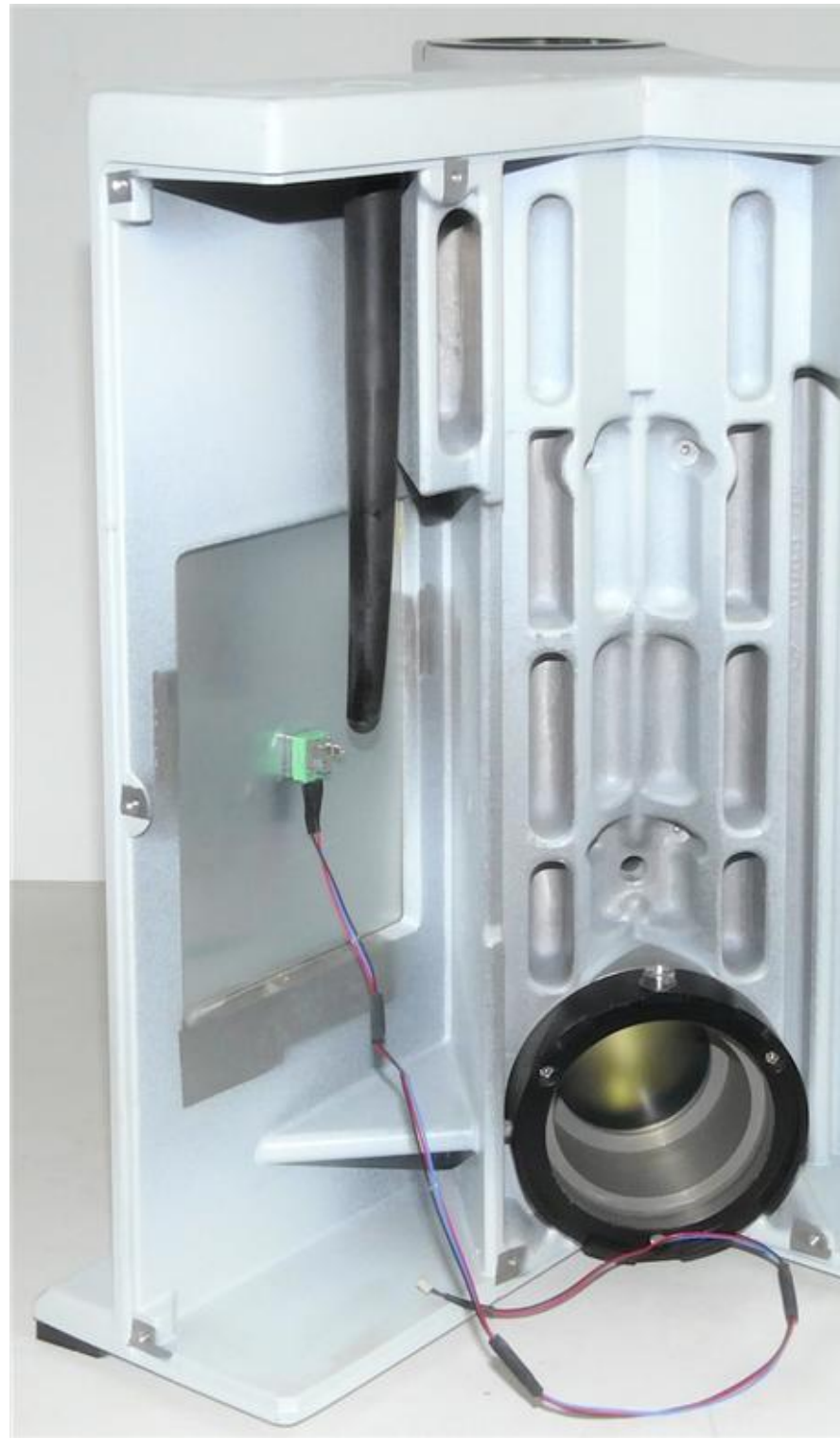
(2) Back view of new adjustment plate with pot and cable.
