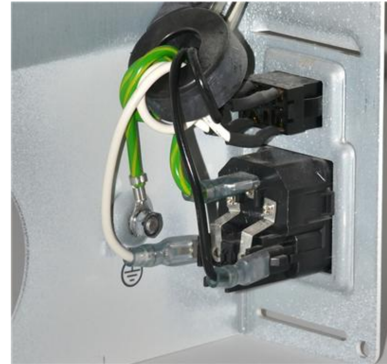
(3) AC power connections at inside of back cover. The white and black leads will be disconnected.
