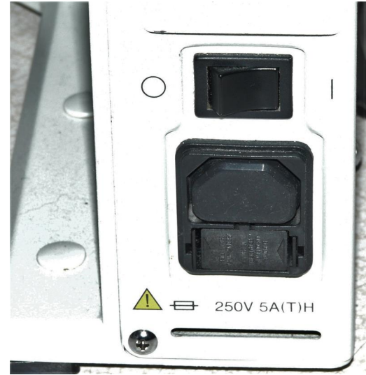
(2) Install PN 10736 rubber plug in AC receptacle to deter connection of AC power.
