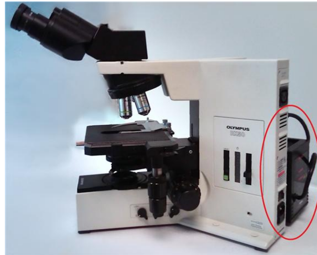
Bottom illuminator for viewing by light transmitted through the sample.
