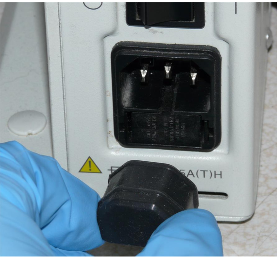
(2) Install PN 10736 rubber plug in AC receptacle to deter connection of AC power.
