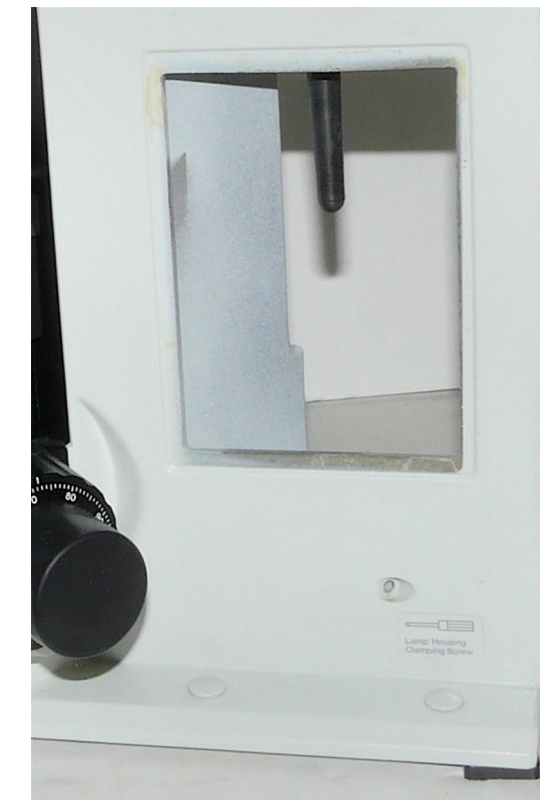
(5) Outside view after removing intensity control plate.
