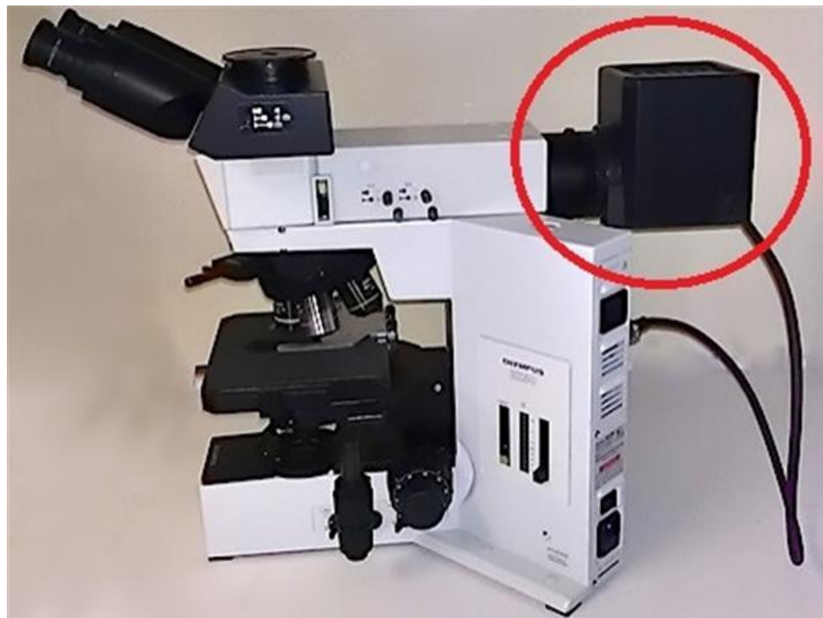
Top Illuminator for viewing the sample by reflected light off the surface.
