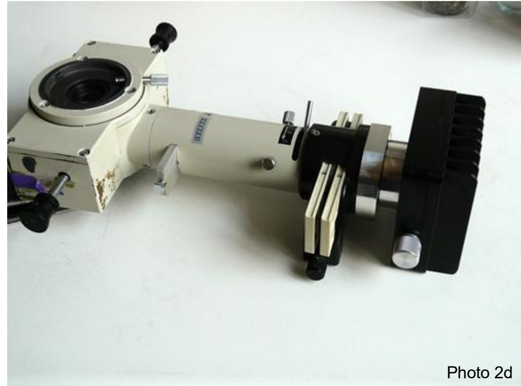
3. Insert the Nanodyne illuminator into the Nanodyne adapter (continued).
