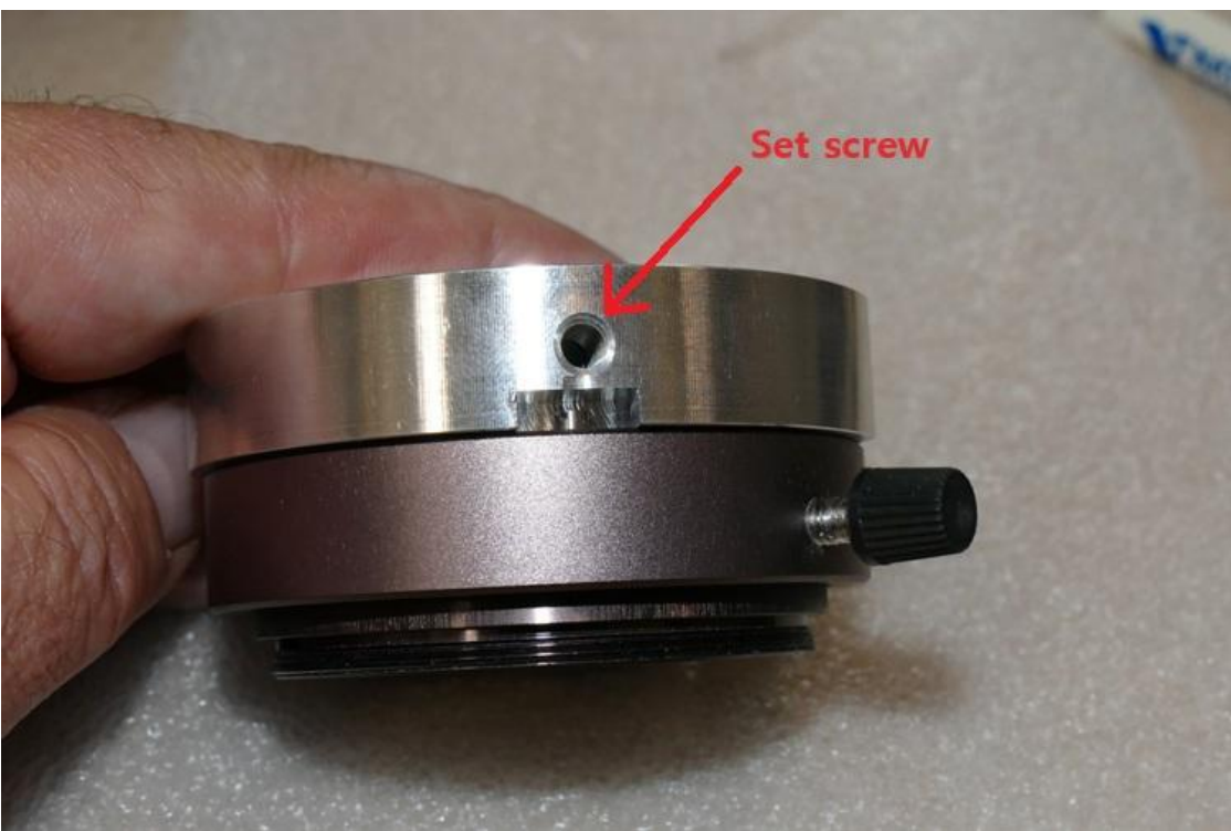
4. Secure the illuminator by tightening the set screw with the 5/64 inch hex key as shown above.
