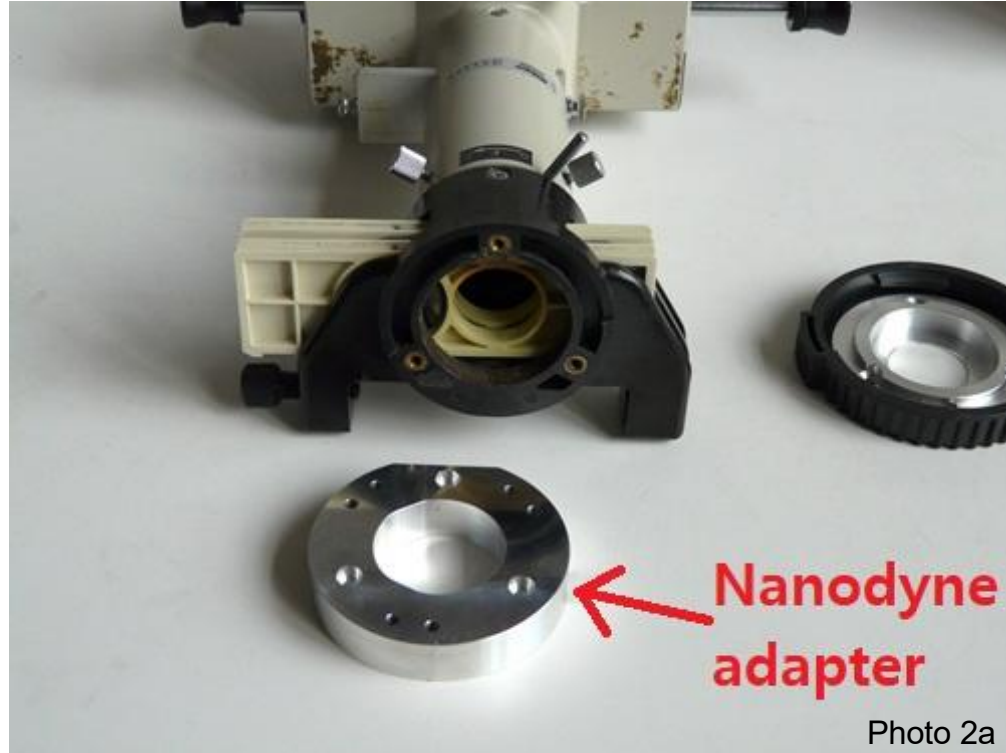
1. Align the Nanodyne adapter with the microscope.
