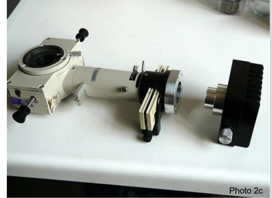
3. Insert the Nanodyne illuminator into the Nanodyne adapter.
