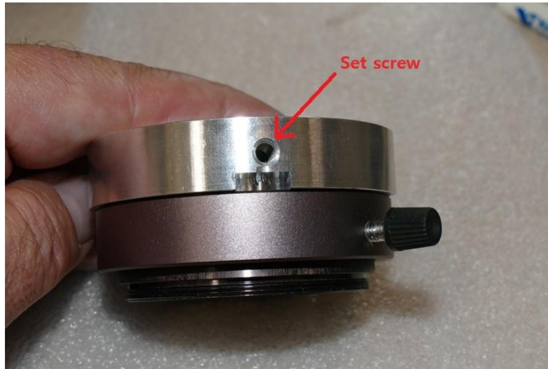
4. Secure the illuminator by tightening the set screw with the 5/64 inch hex key as shown above.
