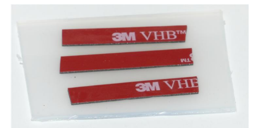
3M VHB tape to secure pot cable
