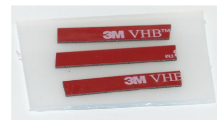
3M VHB tape to secure pot cable
