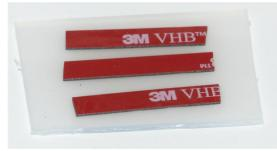
Tape to secure wires.
