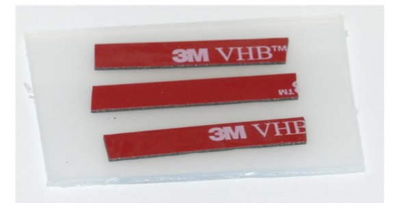
Tape to secure wires.
